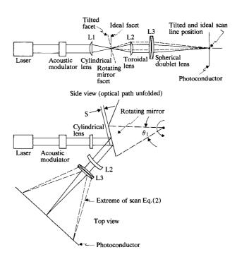
Figure 5 Cylindrical/toroidal lens correction technique.
