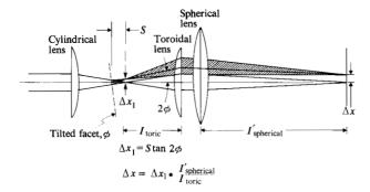
Figure 6 Scan line deflection due to sag S.
