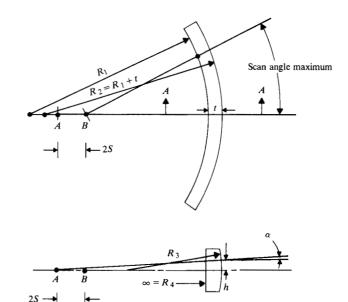
Figure 8 The toroidal lens designed for minimum ray deviation for all scan angles.
