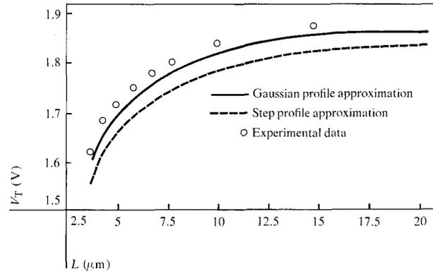
Figure 6  $V_T$  vs  $L$  at  $V_D = 0.1$  V and  $|V_{sx}| = 5$  V.
