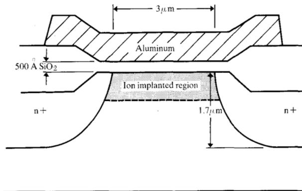
Figure 1 Double-boron-implanted enhancement n-channel MOSFET device structure. Shallow implant concentration is  $6 \times 10^{11}$  atoms/cm<sup>2</sup> at 35 keV; deep implant concentration is  $2 \times 10^{11}$  atoms/cm<sup>2</sup> at 150 keV. Substrate material is 15- $\Omega$ -cm p-type silicon, and substrate concentration  $N_B$  is  $10^{15}$  atoms/cm<sup>3</sup>.
