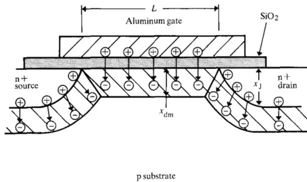
Figure 3 Short channel model structure due to Poon and Yau.
