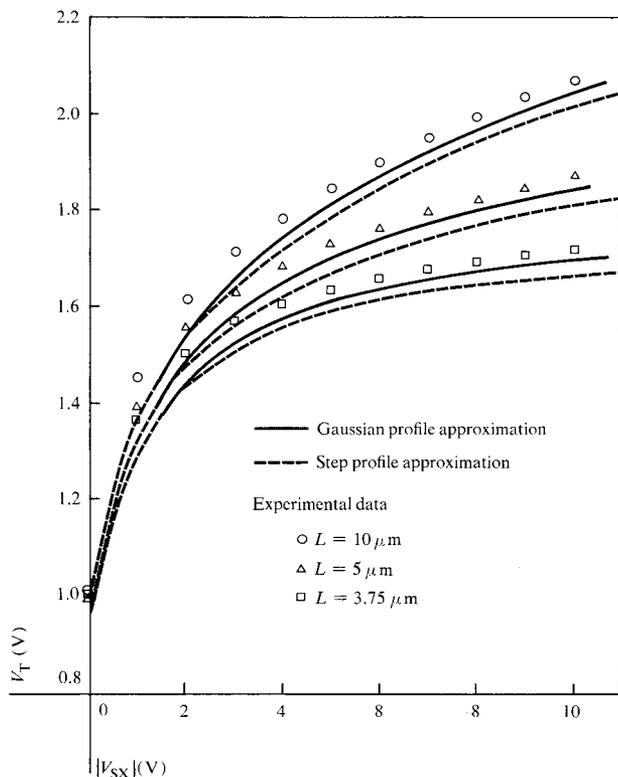
Figure 5 Substrate sensitivity curves of various channel length devices at  $V_D = 0.1$  V.
