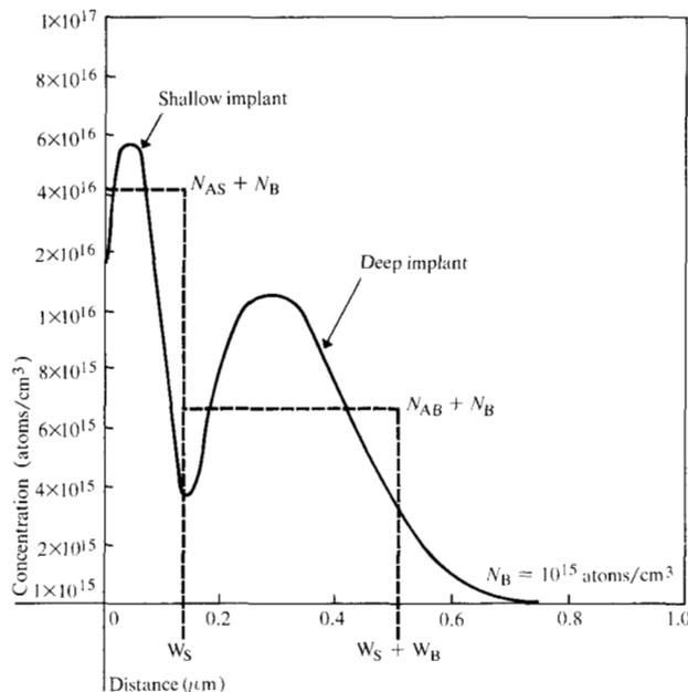
Figure 2 Theoretical ion implant profile and step profile approximation for concentrations given for Fig. 1.
