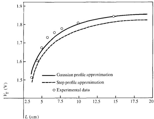
Figure 7  $V_T$  vs  $L$  at  $V_D = 5$  V and  $|V_{sx}| = 5$  V.
