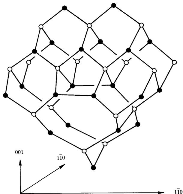
Figure 10 Model of the core of a Lomer dislocation in the sphalerite structure with Burgers vector  $a/2$   $[\bar{1}10]$  and line direction  $[\bar{1}10]$ .
