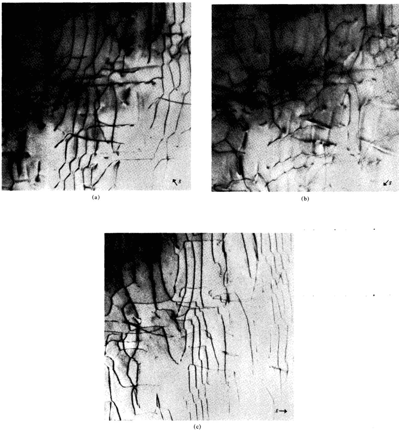
**Figure 5** TEM micrographs of same area as Figure 4, with different diffracting conditions. (a)  $g = [3\bar{1}\bar{1}]$ , extinguishing AC (b)  $g = [1\bar{3}\bar{1}]$ , extinguishing CB, (c)  $g = [2\bar{2}0]$ , extinguishing BA.
