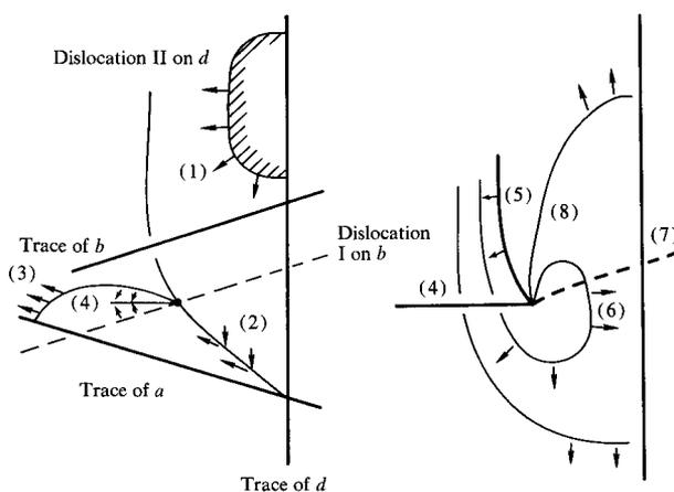
Figure 7 Proposed mechanism for formation of a Lomer dislocation and of a dislocation source.
