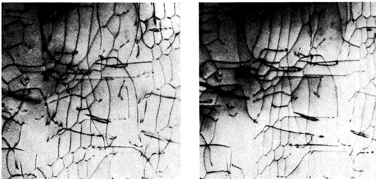
Figure 4 Stereo transmission electron-microscope pair showing networks of elongated dislocation cells (see text).  $g = [2\bar{2}0]$ .  $\times 30\,000$ .
