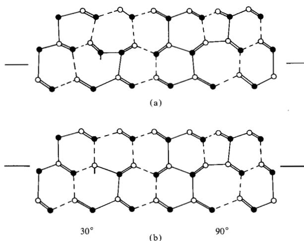
**Figure 1** Dissociated  $60^\circ$  dislocations in the sphalerite structure with  $30^\circ$  and  $90^\circ$  partial dislocations and an intrinsic stacking fault lying between them. (a) Shuffle set; (b) glide set.
