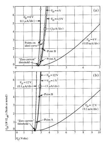
Figure 10 Turn-on characteristics for several current ranges and drain voltages. (a) 500Å device; (b) 1000Å device.
