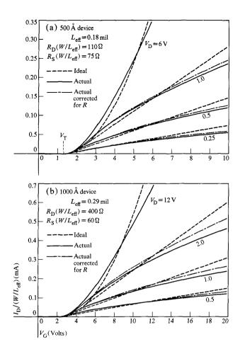
Figure 8 Experimental and idealized transfer characteristics.
