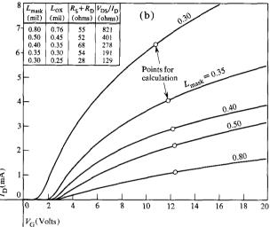
Figure 14 Transfer characteristics for various channel lengths (W = 4 mil). (a) 500Å devices,  $V_D = 0.5$ V; (b) 1000Å devices,  $V_D = 1.0$ V.
