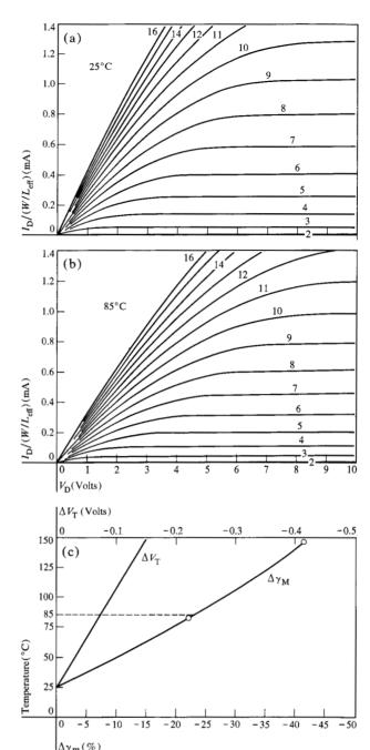
Figure 19 Temperature effects on device parameters for 500 Å device. (a) Grounded-source characteristics at 25°C; (b) grounded-source characteristics at 85°C; (c) threshold voltage and transconductance variations vs temperature.
