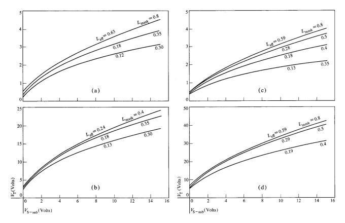
Figure 17 Threshold voltage vs source-to-substrate voltage for various channel lengths. (a)  $500\text{\AA}$ ,  $V_D = 6\text{V}$ ; (b)  $6000\text{\AA}$ ,  $V_D = 6\text{V}$ ; (c)  $1000\text{\AA}$ ,  $V_D = 12\text{V}$ ; (d)  $10,000\text{\AA}$ ,  $V_D = 12\text{V}$ .
