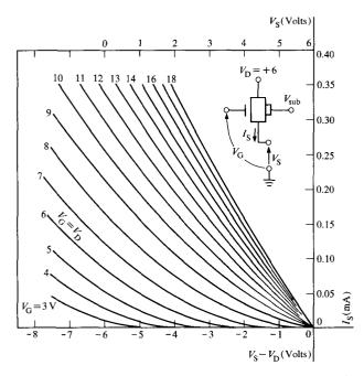
Figure 5 Grounded-drain (load device) characteristics. (500Å device;  $W/L_{eff} = 1/4$ .)
