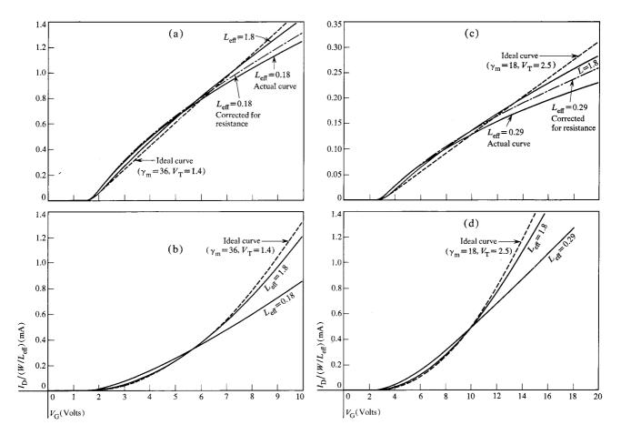
Figure 16 Normalized transfer characteristics above and below pinchoff for long and short channel lengths. (a) 500Å,  $V_D = 0.5V$ ; (b) 500Å,  $V_D = 10V$ ; (c) 1000Å,  $V_D = 1.0V$ ; 1000Å,  $V_D = 16V$ .
