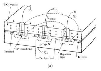
Figure 13 (a) Structure of guard ring using biased n<sup>+</sup> diffusion; (b) leakage current vs substrate voltage for a device with a large surface charge.
