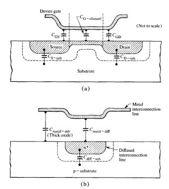
Figure 6 Illustration of (a) device capacitances and (b) interconnection capacitances.
