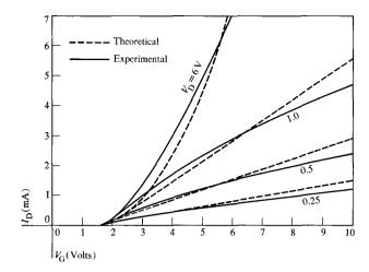
Figure 3 Transfer characteristics of a 500Å device compared with theoretical device equations for constant  $\gamma_m$ . (W = 4 mil;  $L_{\rm eff} = 0.18 \, \text{mil.})$
