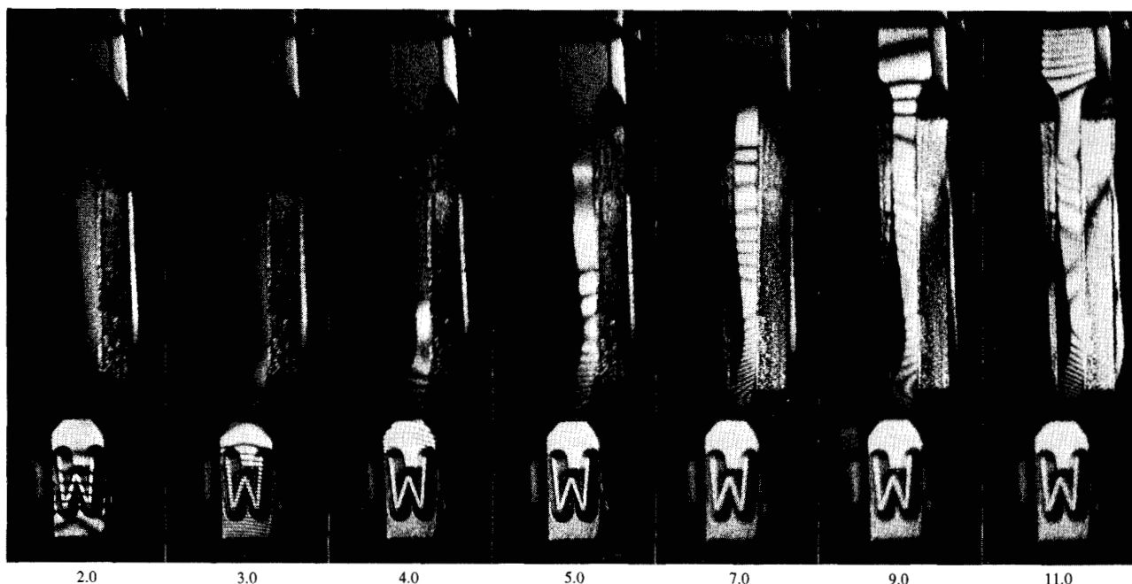
Figure 10 W type-piece, design 1 at 170 in./s, normal alignment. Numbers are T_d in microseconds.
