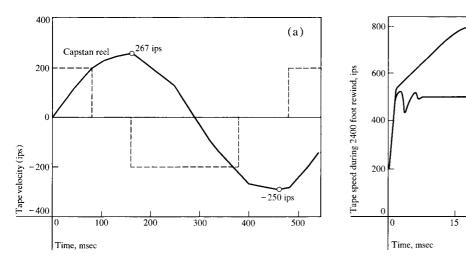
Figure 9 Tape velocity data. (a) Reel speed during worst-case capstan reversals. (b) Rewind speed characteristics.
