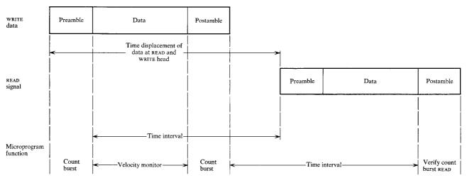
Figure 8 Microprogramming monitor of WRITE data format.
