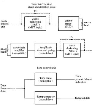
channel diagram, Fig. 10: READ chain, amplitude sense and gating ramp generator, and time sense.
