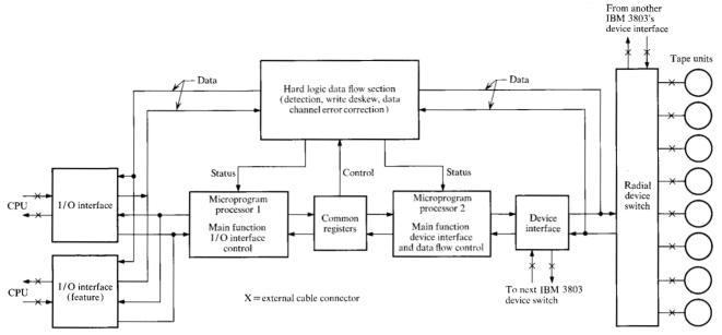
Figure 2 Block diagram of microprocessing.
