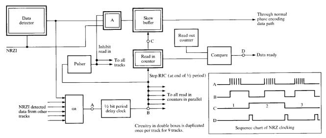
Figure 4 NRZ detection with conversion of NRZ to pseudo-phase encoding.
