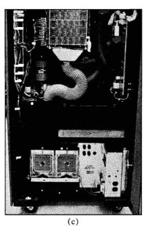
Figure 3 Tape subsystem packages: (a) Front of IBM 3803 Tape Control Unit, showing CE panel at upper left. (b) Rear of IBM 3420 showing cable connector at bottom left; (c) Rear of IBM 2420 Magnetic Tape Unit, showing cable connector and power supply at bottom (for comparison).
