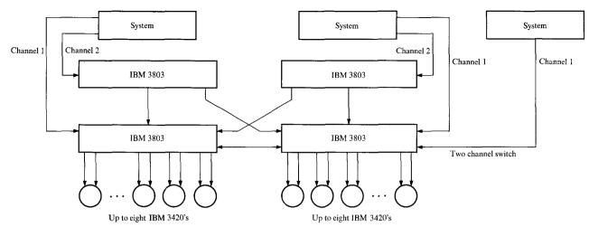
Figure 1 Configuration of the IBM 3803/3420 Magnetic Tape Subsystem showing how four control units communicate with up to 16 tape drives. This example of a typical configuration shows a pool of 3420 drives which can be accessed by three independent systems.
