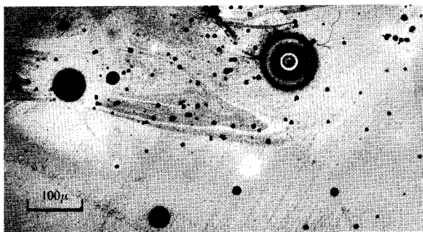
Figure 5 Porosity of the film barriers revealed through chlorine etching.
