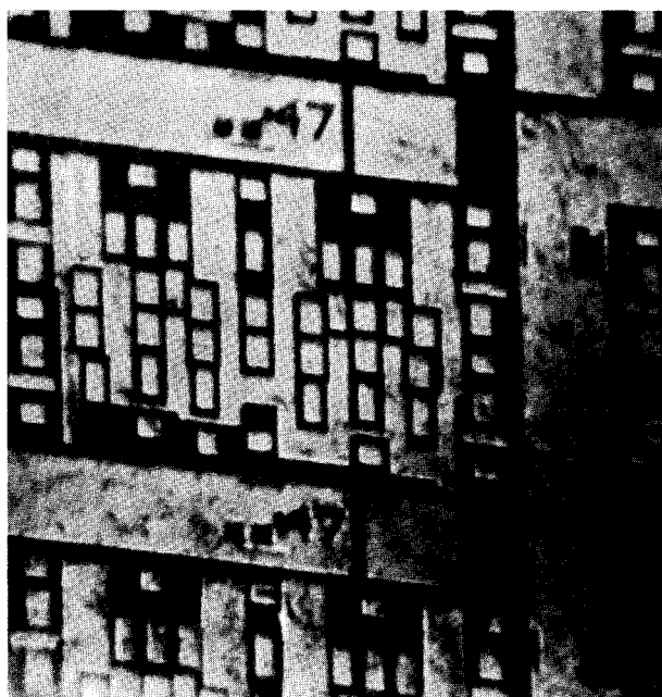
Figure 6 A surface topograph of another wafer section. The test transistor at the top of the figure yielded a leakage current of 240\mu\text{A} as compared with 1300\mu\text{A} for the lower chip. This is consistent with the observed dislocation density in each chip.
