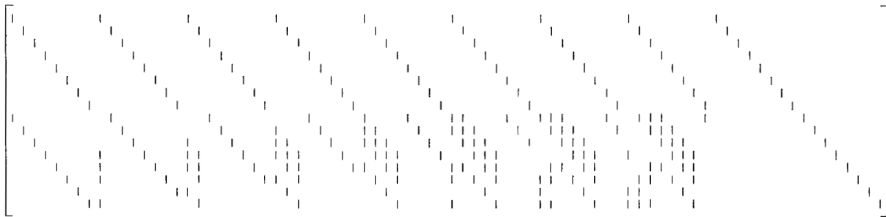
Figure 2 H-matrix for the (80, 64) 8-adjacent-error correcting code.
