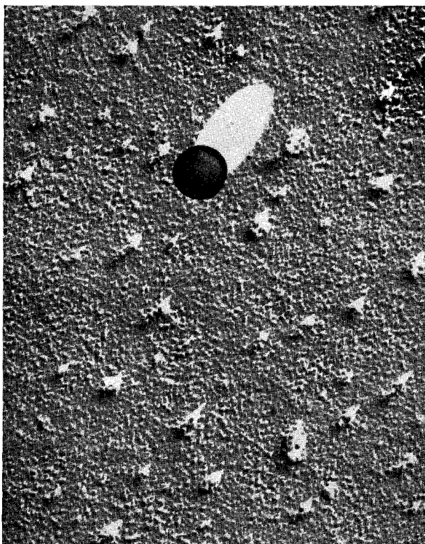
Figure 3 Germanium surface (20,000 \times ) after removal of the heat-treated (16h in vacuum at 800°C) \text{Al}_2\text{O}_3 film.
