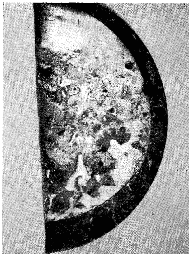
Figure 4 Another Code 823 Cr-Au specimen exhibiting major dewetting after 5 min of immersion in Pb-5%Sn-2% Au. (4.5 \times .)
