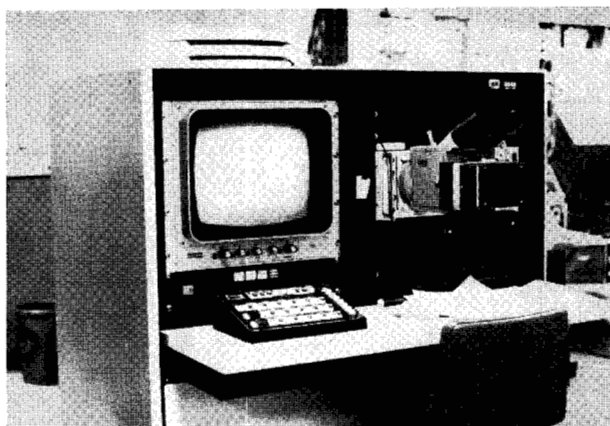
Figure 2 The Yale/IBM Graphics Terminal.
