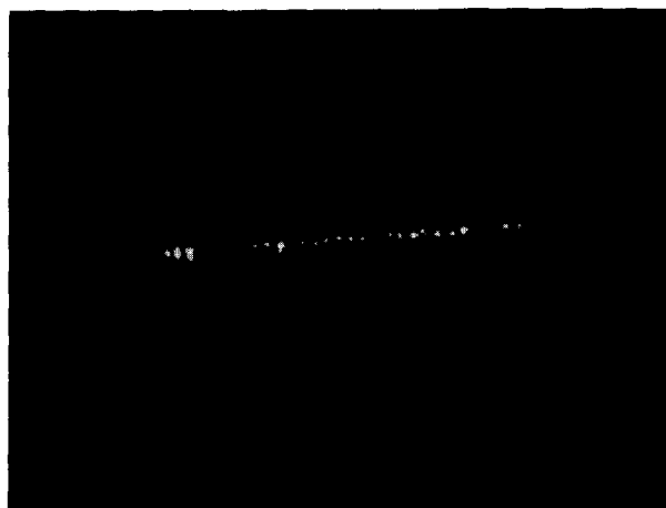
Figure 6 Blanked horizontal sweep 2 cm long. Note nonuniform spot size. Obtained with low-resolution electron gun; resolution was above 60 spots/line.
