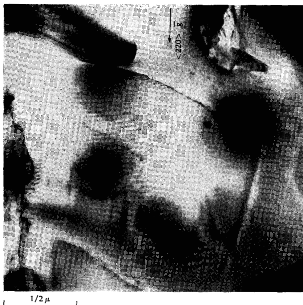
Figure 5 Moiré fringes in the precipitate platelets lying parallel to the film surface. This is a bright field view with a strongly operating \langle 220 \rangle reflection.
