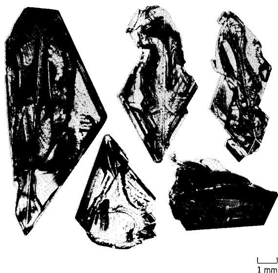
Figure 2 Typical GaP crystals grown from gallium solution.
