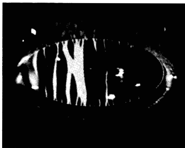
Figure 3 The photograph illustrates the extinction possible for one magnetization state, showing that the reflected light is linearly polarized. The domains are magnetized in the opposite direction.
