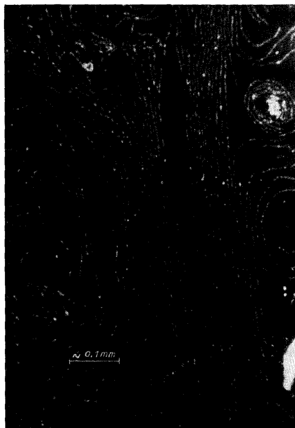
Figure 8 Double Néel walls in a Ni-Fe film with a thickness of about 150 A.
