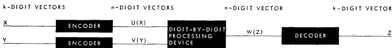
Figure 2 Block coding with digit-by-digit processing.
