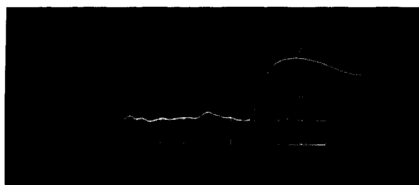
Figure 10 Rise time of the output waveform of the Havens delay unit. A Tektronix Type 517 oscilloscope was used, having a 20-millimicrosecond-per-centimeter sweep speed and a vertical sensitivity of 5 volts per centimeter. The rise time is approximately 8 millimicroseconds.
