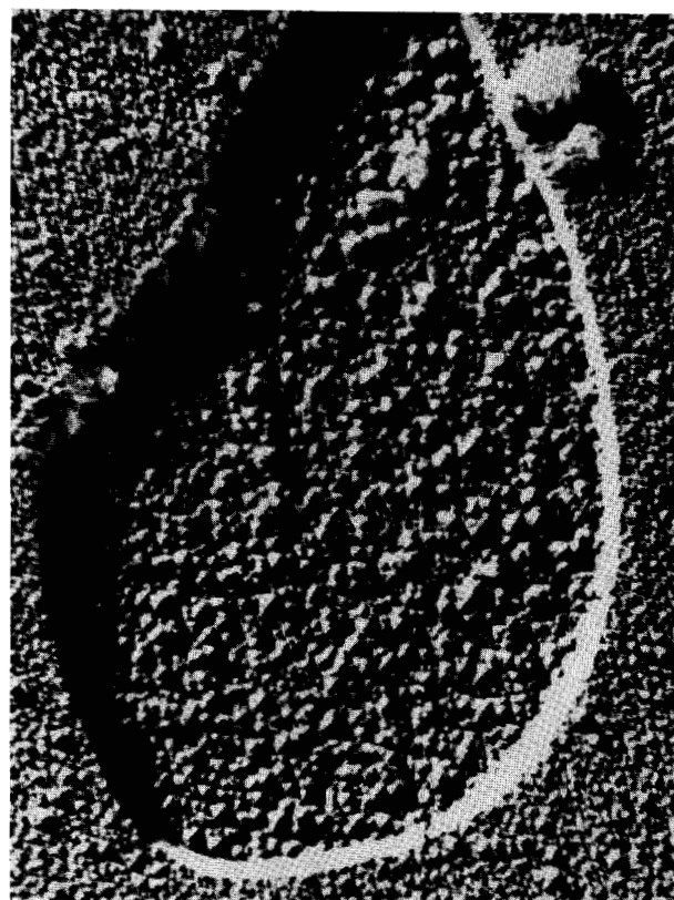
Figure 2 Domain with positive ends of dipoles at surface, surrounded by oppositely polarized domain, 7,000X.
