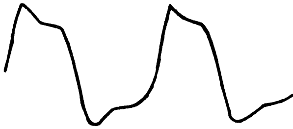
A) 1600 FRPI, OVER-SATURATED
