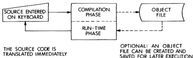
Figure 3-2 Fundamental Incremental Compiler Operation
