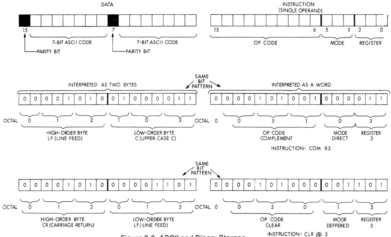
Figure 2-3 ASCII and Binary Storage
