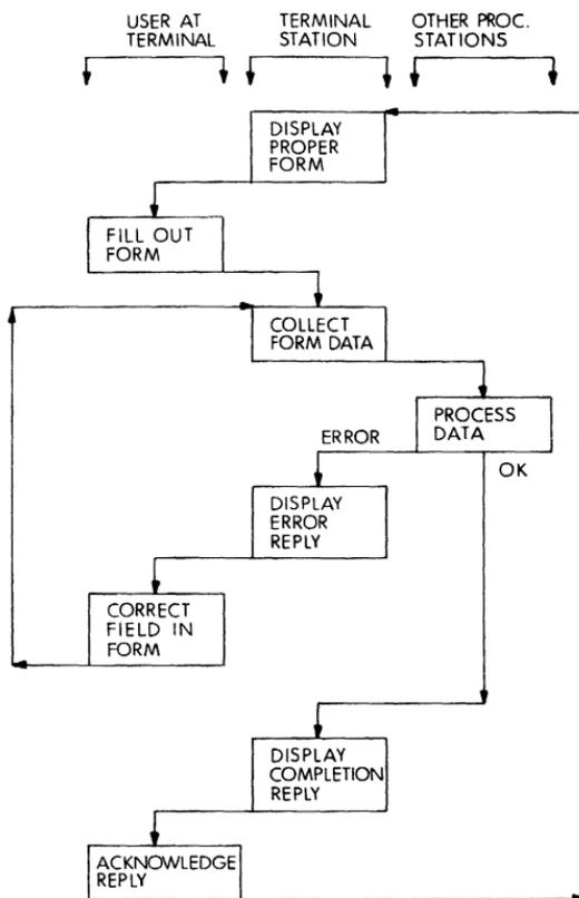
Figure 9-6 Typical Exchange or Message Processing Paths
