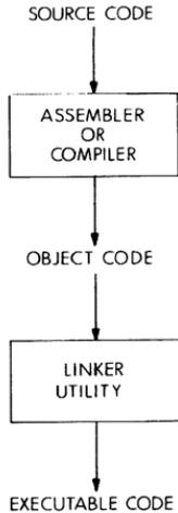
Figure 3-1 Fundamental Assembly or Compilation Procedure
