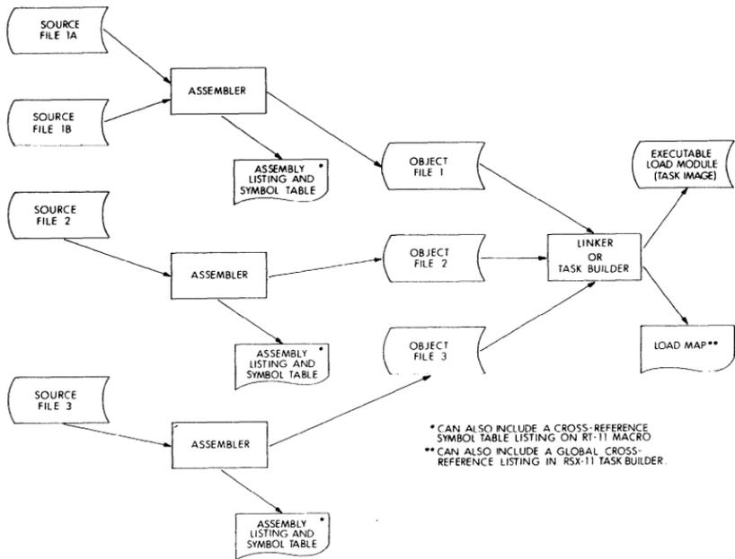
Figure 15-1 MACRO Assembly Procedure
