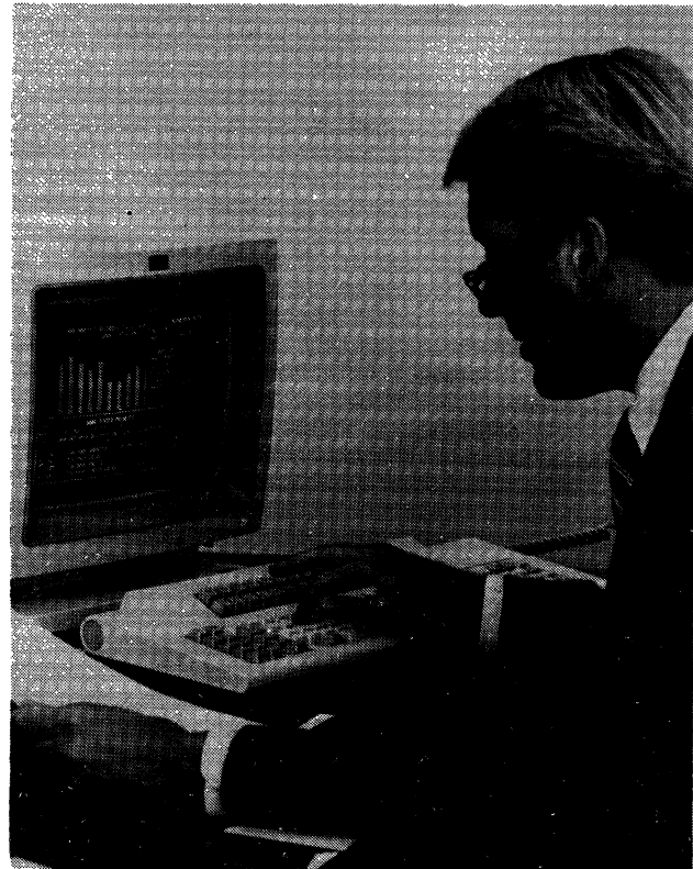
The 3270-PC is a version of IBM's Personal Computer designed for use with the 3270 Information Display System. The key feature of the 3270-PC is the unit's multiple windows—users can operate up to seven concurrent sessions and view them on the screen.
