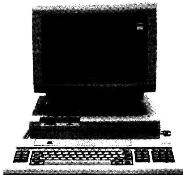
The 3178 Display Station is the replacement for the venerable 3278 display. The 3178 contains an improved ergonomic design, taking up less space than its predecessor. The terminal's modular construction contributes to its ease of use, with a tilt/swivel display and low-profile keyboard.
