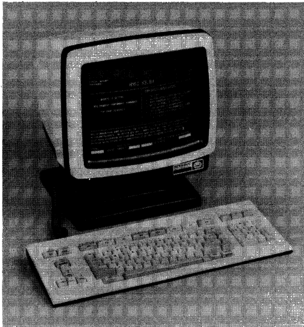
The ATL-008 is the first member of a new family of 16-bit microprocessor-based smart terminals from Beehive. The ATL-008 features a 14-inch tilt-and-swivel monitor, a low-profile detached keyboard, and a display arrangement of 27 lines by 80/132 characters. The ATL-008 is targeted to compete against the ADDS Viewpoint/90 and TeleVideo 970, and is intended as a bridge for Beehive into the desktop microcomputer market.
