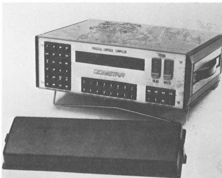
COMSTAR Process Control Compiler. The compiler is designed with all solid state logic, providing high field reliability.
