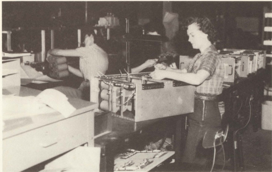
Computer assembly room at the General Electric Computer Department plant in Phoenix, Arizona. This photograph, taken around 1959, shows power supplies being assembled for the NCR-304, which was manufactured by GE. CBI recently learned that most of the records from the Computer Department were destroyed sometime around 1985. This and other photographs of the assembly area were donated by former GE employee, Bill Petterson.
