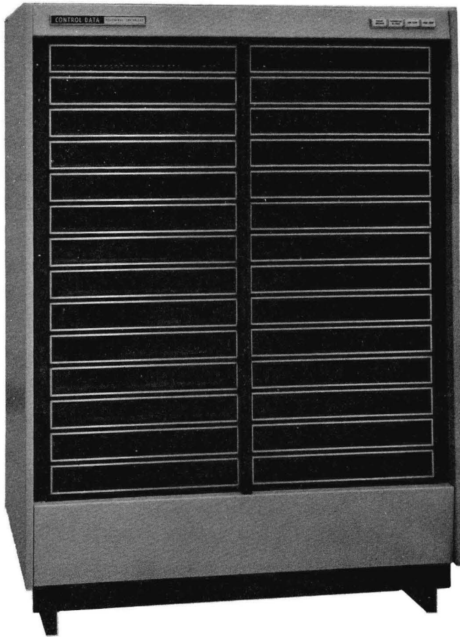
DRUM STORAGE CONTROLLER
