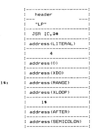
Fig. 3.16 Illustration of DO - LOOP.
