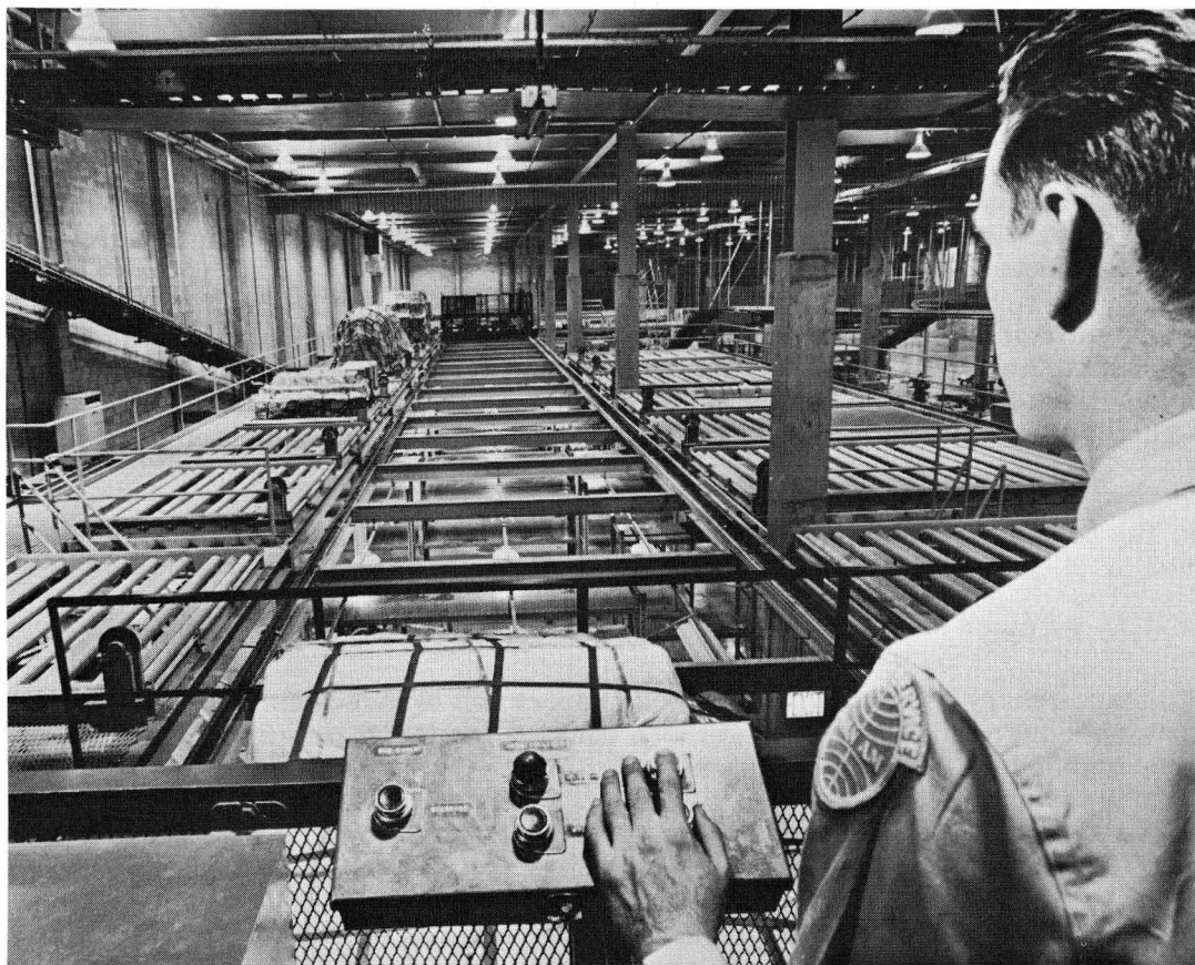
FIFTY-ONE PALLETS, EACH 88 IN. BY 125 IN. , MAY BE STORED IN HOLDING STATIONS AT CARGO TERMINAL.
