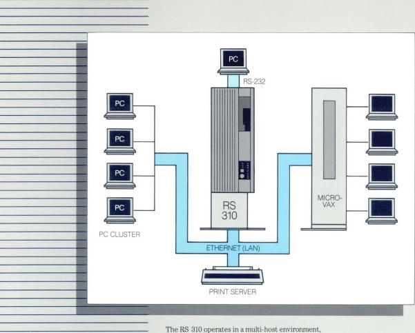
The RS 310 operates in a multi-host environment, allowing for computers of different manufacture to share common data. This multi-host support capability is an exclusive feature of Britton Lee systems.
