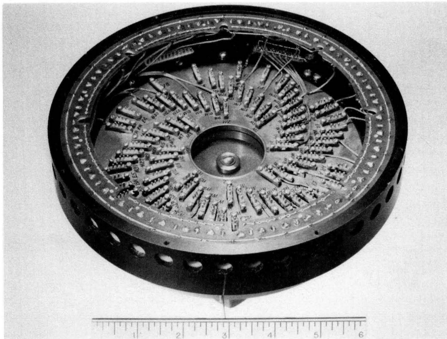
Figure AI-8. RECOMP I Memory, Cover Removed
