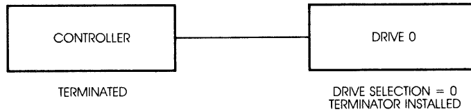
FIGURE 3-3. ONE DRIVE, ONE CONTROLLER TERMINATION EXAMPLE
