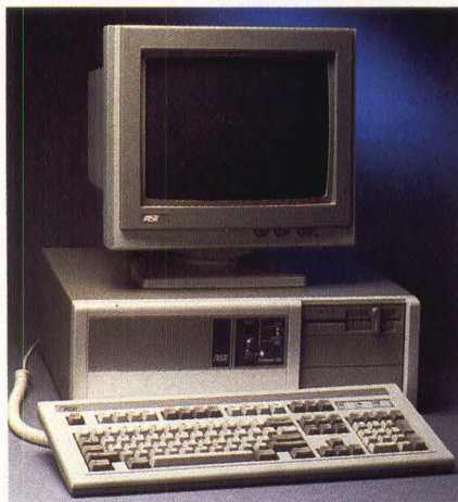
One recent entry in a rising number of PS/2 alternatives is the Premium/386 from AST Research. This system features a 20-MHz 80386 microprocessor, up to 13M bytes of 32-bit static-column RAM, and a 32-bit expansion slot dedicated to memory devices.
