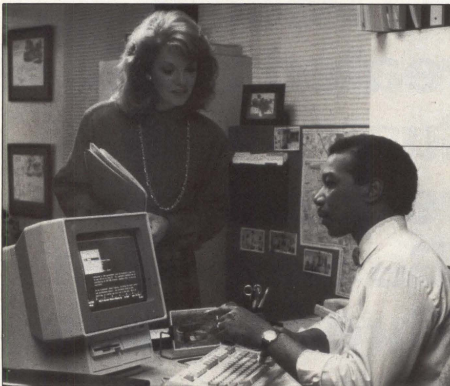
The Personal System/2 Model 25 is touted as a personal workstation that can be connected to an off-site mainframe to download information. It is available with either a color or monochrome display, and two types of keyboards, one compact and the other enhanced for use with other members of the PS/2 family.
