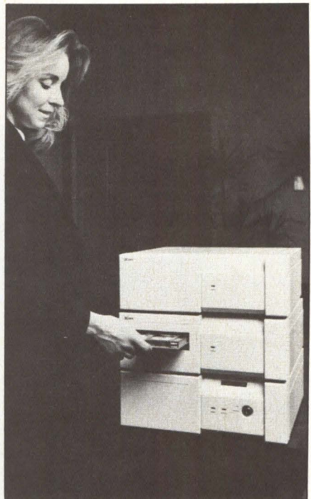
Options: Users can expand 3Server (bottom) with an optional 60M-byte tape-backup unit (center) and 36M-byte expansion disk (top).
