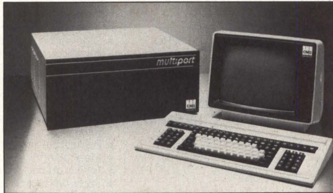
The Multiport II interactive terminal system provides a cluster of terminals and printers with independent and simultaneous access to a variety of host computers and data communications networks.
