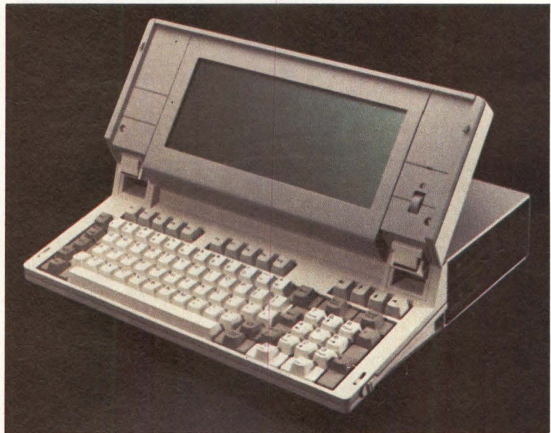
Compact packaging, dual disk drives, a 25-line, 80-column liquid crystal display and MS-DOS and CP/M-86 distinguish International Quartz's 9242 transportable.
