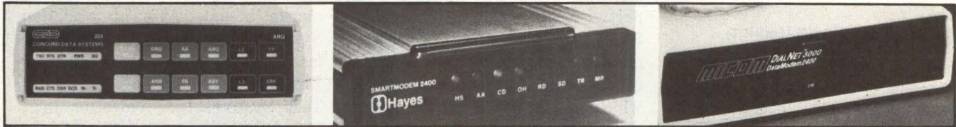
Three new entrants into the full-duplex, 2,400-bps modem market, from left, the $1,295 Concord Data Systems 224, the $899 Hayes Smartmodem 2400 and the $895 Micom Dial Net 3000.
