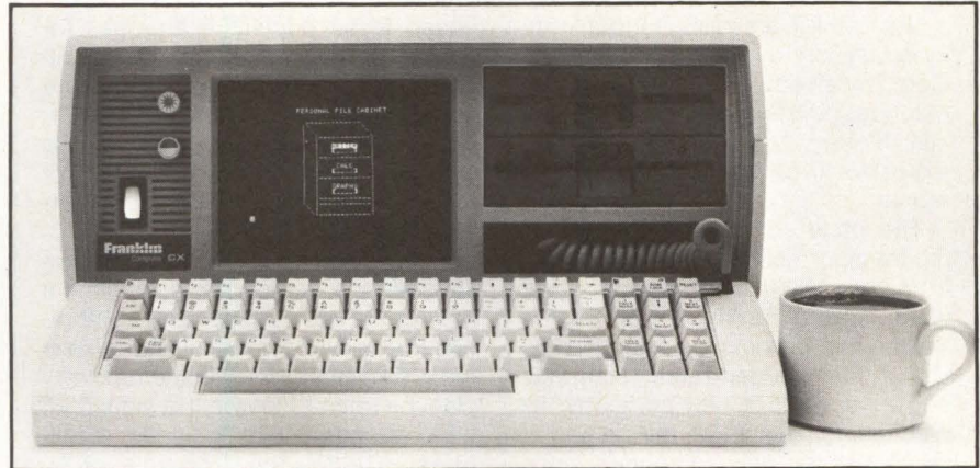
Franklin Computer Corp.'s 27-lb. CX computer is the first portable to run Apple II software, MS-DOS and CP/M. However, Franklin is strapped for funds and may not be able to produce the CX in quantity.
