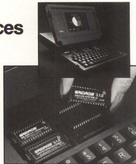
Grid's Compass II offers as much as 1.4M bytes of solid-state memory, including 512K bytes of RAM, 384K bytes of bubble memory and as many as four 128K-byte ROM cartridges. Grid is offering a ROM cartridge with software that emulates IBM 3101 and 3270 terminals, among others.
