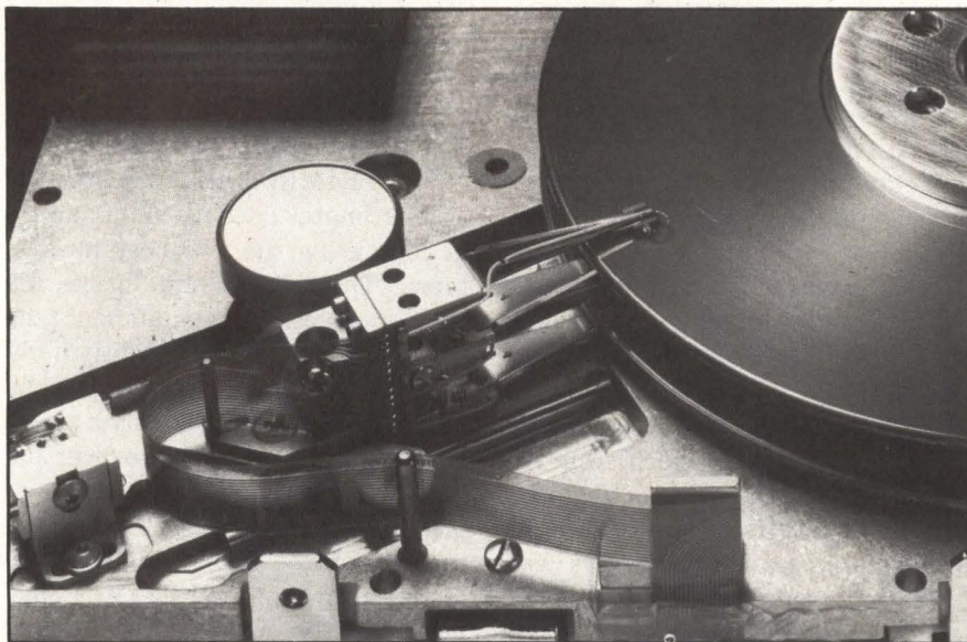
Measuring 1.6-inches high and packing 25.52M bytes of unformatted storage on two platters, the Cogito PT925 Winchester drive is plug-compatible with systems using ST412 controllers.
