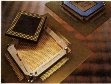
A variety of housings for ICs are making them easier to place in any design. Higher pin counts, increased packing densities, and the use of surface-mount technology make specialized IC packages viable options to the standard DIP (pg 63).
