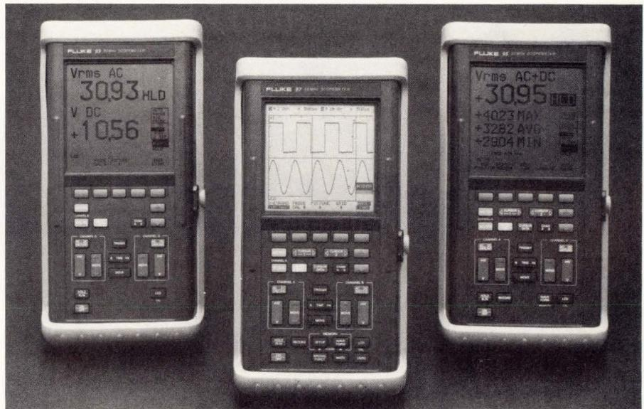
*With displays that occupy about one-third of their area, the 90-series Scopemeters look a bit unconventional. The combination of a 50-MHz, 2-channel DSO, a full-function DMM, and a function generator in a handheld, battery-powered instrument is even more unconventional.*
