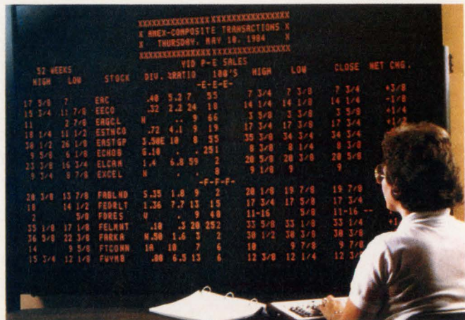
Fig 1 —This 40×64-in. gas-discharge display panel includes 48 modules from Displays Inc. Each module contains two 20-character rows of 1.0-in.-high characters.
