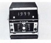
**DC VOM** has five ranges of dc volts with 100  $\mu$ V resolution, and five ranges of ohms with resolution of 0.1 $\Omega$ . Basic accuracy is 0.1% of reading. Model 261 has both self-check zero and calibration front-panel controls. It is available with battery pack for complete portability. Price is \$279 and availability is stock to eight weeks. United Systems Corp., 918 Woodley Rd., Dayton, OH 45403. **209**
