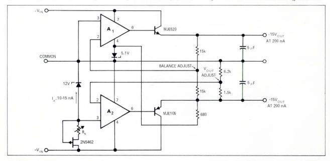
Fig. 6-Single reference source and feedback network to  $A_2$  provide regulation of the negative output. The positive output tracks the negative in this balanced regulator. The outputs can be balanced to within millivolts of each other or can be offset.
