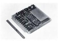
**CORE MEMORY MODULE,** Model 620, is a 1024-word by 10-bit configuration that fulfills desk-top computer and similar smallmemory requirements. Operational modes are full-, half- and split-cycle. Access time is 350 nsec and the cycle time is 1  $\mu$ sec. The unit operates over the 0 to 60°C temperature range and is nonvolatile. Fabri-Tek, Inc., 5901 S. County Rd. 18, Minneapolis, MN 55436.
