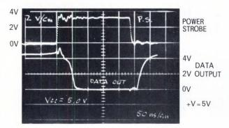
Fig. 4 – In the dynamic operation of a M $\mu$ L 4106, the power strobe to data output delay is 50 nsec with power switching (see scope trace) and 30 nsec without.
