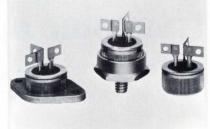
CENTER-GATE, GLASS PASSIVATED TRI-ACS are rated at 30 and 40A, and provide improved dv/dt and di/dt characteristics. Passivation is done with a very dense, void-free sodium-free glass that provides a hermetic seal and eliminates "punchthrough". They are available with  $V_{DROM}$  ratings from 50 to 600V, and in press-fit, studmount and TO-3 packages or chip form. Hutson Industries, 2019 W. Valley View Lane, Dallas, TX 75234. **200**
