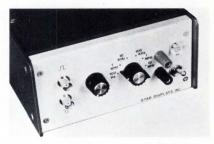
PULSE GENERATOR/POWER SUPPLY was expressly designed for display and TTL circuit checkout. Power output is 5V at 2.5A dc, regulated and short-circuit proof. Pulse output is either positive or negative pulse trains from 30 Hz to 10 MHz. Size of the unit is 3-1/2 by 7 by 7 inches. Star Displays, Inc., 1655 W. 11th Ave., Eugene, OR 97402. **212**
