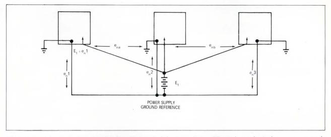
Fig. 7–Common power supply used with independently grounded units results in a differential ground noise between power-supply ground reference and each major unit ground. This is caused by the ground noise differential between each major unit ground.
