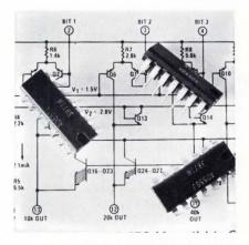
IC QUAD CURRENT SWITCH, Model AD550, is offered in sets of 2 or 3 switches designed for 8- or 12-bit D/A converters. Switching time is 500 nsec, and settling time (to  $\pm 1/2$  LSB) is 1.8  $\mu$ sec for 12-bit sets. Price is \$6.00 for the 8-bit set in quantities of 1000. Analog Devices, Inc., Route 1 Industrial Park, Box 280, Norwood, MA 02062. **204**
