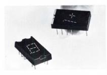
GAASP LED READOUTS, Types 745-0003, 0004 and 0006 have 0.270-inch characters. Each is available with a seven-segment digit or with a  $\pm 1$  symbol. They are rated for 30 mA continuous forward current/segment. Maximum reverse voltage is 6V and peak light emission is at 650 nm. In orders of 1000 or more they are priced at \$7.50 each. Dialight Corp., 60 Stewart Ave., Brooklyn, NY 11237. **172**
