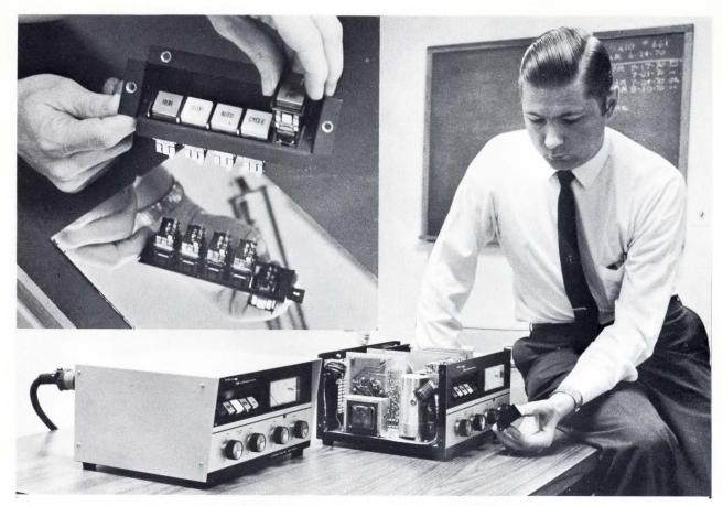
Fig. 2-The switches are Licon type-16 units. They have singlepole, double-throw contacts rated at 10A. They snap into a subas-
