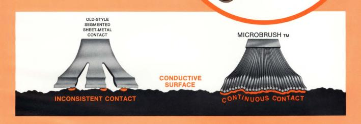
A fully self-conforming contact like MICRO-BRUSH provides —
