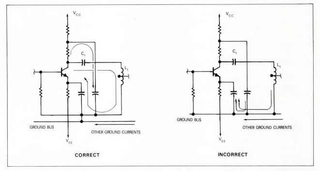
Fig. 5 – **Ground connections for plug-in units** are important considerations in order to prevent built-in noise paths. As shown here, all grounds within any stage should be tied to a common point before being tied to the common ground line.
