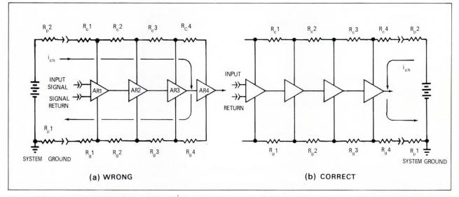
Fig. 4–**Right and wrong power and ground distribution methods** are shown for cascaded amplifier stages. The impedance between the circuit board connector and the power supply is also shown, because in a typical system the distance from a printed wiring board connector to the power source is much greater than the distance between the connector and the stage farthest removed from it on the board.
