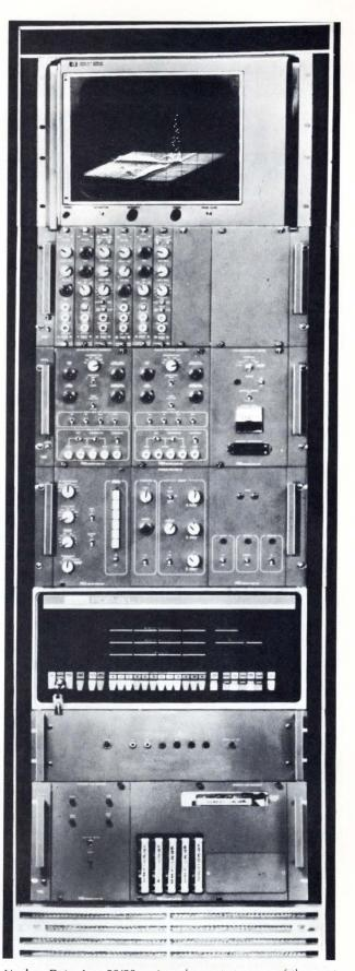
Nuclear Data, Inc. 50/50 system demonstrates one of the most fundamental forms of softcopy computer graphics – point plot in three dimensions. This type of system usually employs a small computer, in this case a PDP-8/L.
