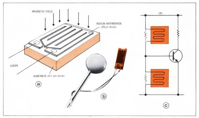
Fig. 1-Magnetoresistors typically are etched into serpentine patterns (a and b). A perpendicular magnetic field will increase their
