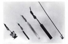
**THERMAL-RIBBON TEMPERATURE SEN-SORS** provide sensing of temperatures from –328 to +500°F. Two basic sensor types are available: Platinum or nickel-iron element resistance thermometers, or lower cost thermocouples. Suitable for sensing of air, gas, liquid or solid surface temperatures, they are available with or without a selfadhesive strip for press-on installation. Minco Products, Inc., 7300 Commerce Lane, Minneapolis, MN 55432. **180**
