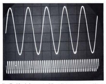
Versatility of the gain-phase meter is well-illustrated by its ratio-measuring capabilities. It can measure, in dB, the log ratio of two signals. Further, these signals need not be of the same frequency, which increases the instrument's usefulness.
