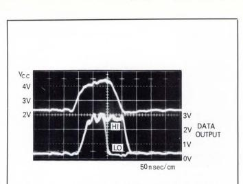
Fig. 8-**Top trace** is  $V_{cc}$  pin at the 93400 with a 2V standby, and the bottom trace is the input/output data line reading out a checkerboard pattern. A tester verified the checkerboard pattern accuracy. Note that the unselected state of the data line is low because  $V_{cc}$  falls below 3V in standby. Because of the power switch circuit delay and the reduced operating value of  $V_{cc}$  due to  $V_{sat}$  of Q1, the 93400 read data access time is increased by approximately 70 nsec.
