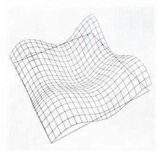
Three-dimensional surface plot is an example of hardcopy computer graphics. Using a FOCAL-based plotting program, this was generated with a PDP-8/L computer. Because of the program elements, this sort of plot is usually not performed in softcopy. If it is, then it is generally generated on a storage tube.
