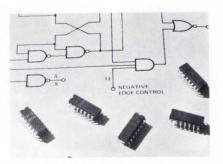
**BIDIRECTIONAL ONE-SHOT IC,** Type N8T20B, triggers on either positive or negative pulse edge, or both. Designed for processing of high-speed, low-level digital signals, it functions as a zero-crossing detector with thresholds of  $\pm 4$  mV. Output pulse width can be set from 10 to 800 nsec,  $\pm 1.0\%$ . Price is \$5 per unit in orders of more than 100. Signetics, 811 E. Arques Ave., Sunnyvale, CA 94086. **203**
