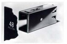
**REAR PROJECTION READOUT** provides 48 discreet messages. The unit is about 3 inches long by 1-1/3 by 3/4 inches and weighs just over 3 oz. The readout, designated Series 1002, has resolution adequate to permit messages of up to four lines of eight characters each to be projected in seven point type size. Quantity pricing of the Series 1002 is \$82 each. Industrial Electronic Engineers, Inc., 7720-40 Lemona Ave., Van Nuys, CA 91405. **174**
