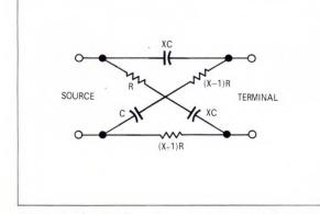
Fig. 1 – Lattice configuration offers better performance than other passive-component selective filters. Factor X should be 10 or larger.
