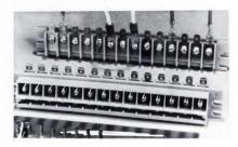
TERMINAL BLOCK accepts PC cards. Multi-tap printed circuit edge connector accepts 0.062-inch-thick single-side printed circuit cards at base and provides terminal block connections for wiring on top. It is available in 14 or 16 position sizes with conductors on 0.375-inch centers. AMP Inc., Harrisburg, PA 17105. **173**
