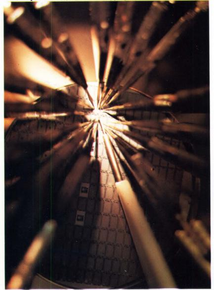
The first pilot wafer of Signetics Corp.'s 1024-bit bipolar RAM is shown during wafer probe testing. This memory device em-
