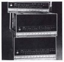
THREE COMPUTERS, 1210, 1220 and 820, are the latest members of the Nova family. The 1210 costs \$4350 with 4k of core memory and \$5750 with 8k words. The 1220 with low-cost expansion capability is priced at \$5250 with 4k memory and \$6650 with 8k. Both have cycle time of 1200 nsec. The 820 with an 800 nsec cycle time is priced at \$6450 (8k memory) and \$7850 (8k memory). Data General Corp., Southboro, MA 01772. **161**
