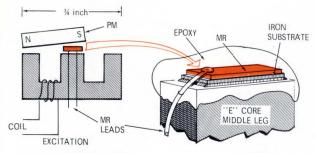
We found that small permanent magnets would produce 10% increases in resistance and that stronger magnets such as the types used in ordinary small speakers would raise the device's resistance from 500 $\Omega$  to 1k $\Omega$ . Half an ampere through the approximately 100-turn coil would produce a 3% change in resistance. It was important, we noted, to concentrate the magnetic flux across the MR by bringing the north and south ends of the magnet up close to the "E" core legs.
