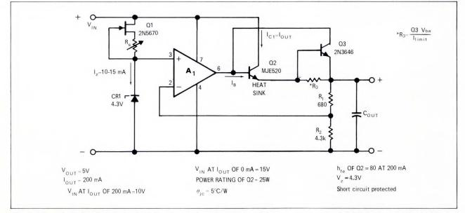
Fig. 3-IC regulator circuit includes short-circuit protection. The reference voltage is chosen to be slightly less than the output voltage.
