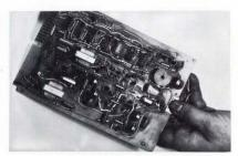
**COMMUNICATIONS CONTROL MOD-ULES, LINE-CONTROL MODULE,** Model 906013, and "handshake" module, Model 906008, can be employed in either tone (DTMF) or rotary dial pulsing applications. Both modules are on a 5.5- by 8- by 1-inch card. For small quantity orders, unit prices are \$155 and \$112 respectively. G-V Controls, Div. of Sola Basic Industries, 101 Okner Parkway, Livingston, N J 07039. **160**
