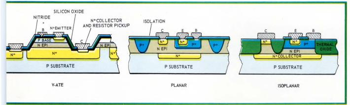
Both the Isoplanar and V-ATE (vertical anisotropic etch) processes, developed by Fairchild Semiconductor and Raytheon Semiconductor respectively, are more complex than the standard Planar process, but they result in reductions of as much as 60 percent in memory cell area.
