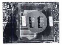
TTL QUAD 2 NAND BUFFER ICs drive highly capacitive loads. The "7437," can drive three times the load of a "7400." Similar to the "7403," the "7438" has opencollector outputs to permit "wired-AND" applications. Propagation delay time is less than 15 nsec low to high. The plastic N7437A costs \$0.78 each, and the S5438F (KOVAR DIP) \$5.04 each in 100 quantities. Signetics Corp., 811 E. Arques Ave., Sunnyvale, CA 94086. **197**
