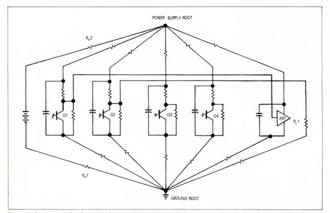
Fig. 2–Single-point ground and power-feed system eliminates noise paths between stages that exist through power supply and ground leads. The power supply source resistance and the line drops must be kept as small as possible.
