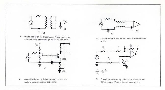
Fig. 3 - Various ground isolation systems can be used to isolate signals between units from their common ground systems.
