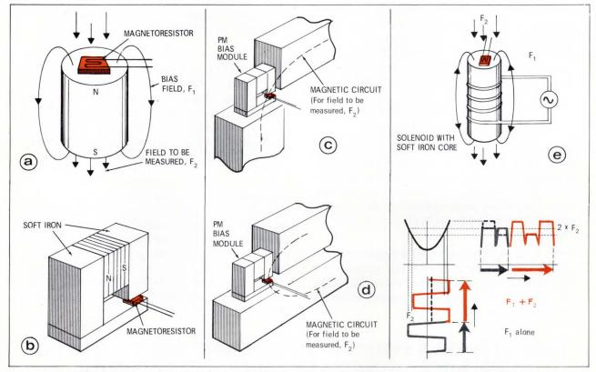
Fig. 4 – Magnetic Bias for MR's improves both their sensitivity and linearity. It is not difficult to accomplish with either small perma-
