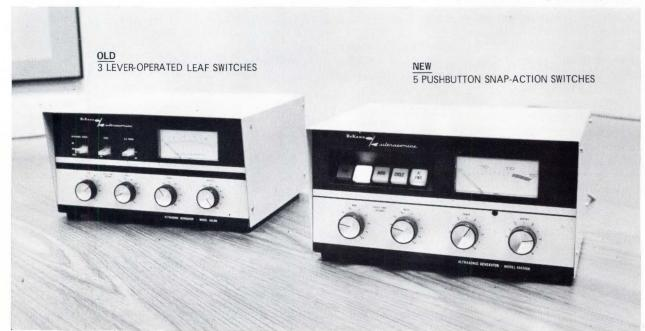
Fig. 1-The redesigned front panel (right) does not look much different than it did before the redesign (left). But the five new
