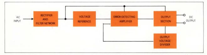
Fig. 1 – Feedback voltage regulators are made up of these basic building blocks. An IC op amp can be used as the error detector.
