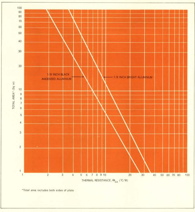
Fig. 4 – Heat-sink area is determined for bright or black anodized aluminum from the calculated value of  $\theta_{sa}$ .
