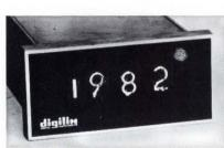
**DIGITAL DISPLAY** designed for direct connection to current and voltage transmitters is available in 3-1/2- or 4-digit versions. For applications where transmitter output is not linear with respect to the input, a nonlinear A/D converter is available. Standard TTL-compatible BCD output is accessible at the rear panel. Price is from \$169 up, depending on configuration. Digilin Inc., 1007 Air Way, Glendale, CA 91201. **177**
