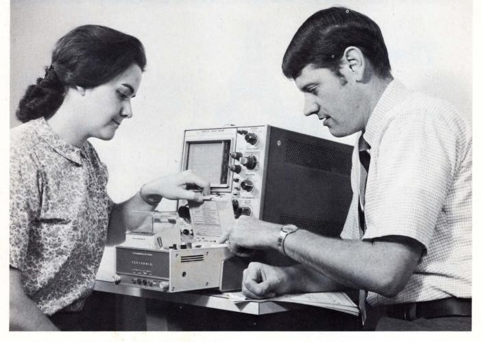
With the 172 Programmable Test Fixture for the TEK-TRONIX 576 Curve Tracer, you program up to eleven sequential tests on FETs, transistors and diodes. This new fixture saves measurement time in applications such as incoming inspection where you make a series of tests on a number of devices.
