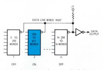
Fig. 2 - Only one memory package operates when the data output line is in a wired AND connection. For example, if word 389 is addressed, only package 2 is in an operating mode. For this configuration, the OFF (reset state) is a high-voltage level.
