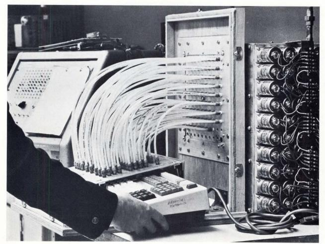
The most sophisticated part is the control and error checking unit. When evaluating a completed keyboard, the control unit activates each solenoid consecutively – which, in turn, directs a small burst of air to the desired key. The ASCII output from the keyboard under test is compared with a valid unit and all errors are displayed. A lamp panel contains one lamp per key and accommodates up to 100 keys.
