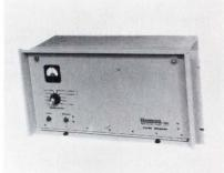
ONE WATT, 12 GHZ MICROWAVE RA-DIO for CATV CAR band distant signal relay use, Model MA-12G, is entirely solidstate. The unit is intended for wideband video use in the 12.7 to 12.95 GHz band. Transmitter section features a 2 GHz crystal oscillator with 0.005% stability, while the receiver is a super-heterodyne with 70 MHz IF and a GUNN-diode local oscillator. Microwave Associates, Inc., Burlington, MA 01803. **213**
