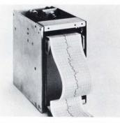
**STRIP CHART RECORDER** uses fan-fold paper. Model GRZ-70 features front paper loading, rectilinear hot-stylus recording and a choice of one to four speeds. Primarily intended for OEM use with electrocar-diograph and fetal monitoring equipment, the unit is available with single and dual 50 mm channel configurations as well as a dual channel of 50 and 80 mm. General Scanning Inc., 80 Coolidge Hill Rd., Watertown, MA 02172. **210**
