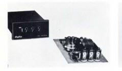
**DPMS FOR OEM USE** feature automatic polarity detection, 0.6-inch gas-discharge display tubes and standard TTL-compatible BCD output. Measuring range is 0 to  $\pm 1.999V$  including overrange. Model 1352 (without case) is priced at \$125 and Model 2352 (with case) is \$159. BCD option is \$15 extra. Digilin, Inc., 1007 Air Way, Glendale, CA 91201. **206**
