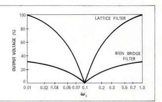
Fig. 2–**Note the improved selectivity** and greater output voltage of lattice filter compared with that for Wien bridge.
