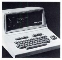
**VIDEO-DISPLAY TERMINAL,** Model 401, features a 132-character display consisting of four lines of 33 characters each. A  $5 \times 7$ dot matrix forms a 63-character USASCII code. There are indicators for operator control and six special functions. The basic unit is adaptable to a variety of off-line and online configurations. Single unit prices begin at \$1495. Centronics Data Computer Corp., 1 Wall St., Hudson, N H 03051. **155**
