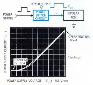
Fig. 1–A power strobe enables the power switching circuit connected between the power supply and the V<sub>cc</sub> of the bipolar ROM M $\mu$ L 4106. Operating and standby bias points are indicated on the scope trace (I<sub>cc</sub> vs V<sub>cc</sub>).
