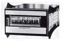
SIX-DIGIT IMPULSE COUNTER that features snap-in mounting, requires only 1.2 by 2 inches of panel space. Reliability is rated at up to 250 million counts. Standard options include manual or electrical reset, internal illumination and reverse-color wheels. Count speeds are up to 100/sec. Price is \$21.30 each in lots of 100. Kessler-Ellis Products Co., Atlantic Highlands, N J 07716. **178**
