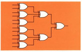
MC10160 12-Bit Parity Generator/Checker. Useful for high speed detection or generation of parity on long data words with minimum package count. One package offers nine EXCLUSIVE-OR gates internally connected to provide odd parity checking or generation.
