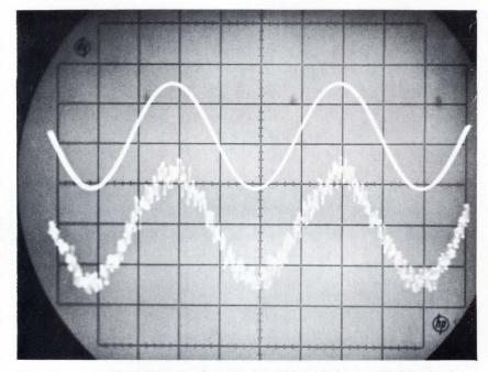
**Phase measurements of noisy signals** are readily made with the new 3575A gain-phase meter. Even the high-frequency noise present on the lower trace does not preclude a useful phase measurement, for it only results in a phase offset of 2.5° – and the measurement is free of jitter or bobble in the readout.
