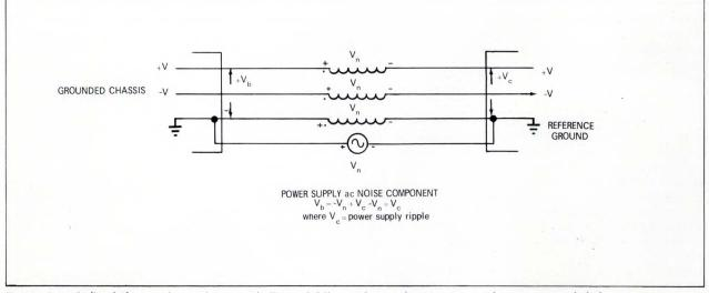
Fig. 6-A 3-winding balun can be used to cancel effects of differential ground noise on a unit having a grounded chassis.
