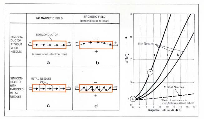
Fig. 2-**Sensitivity of MRs** can be much improved by embedding nickel needles that are aligned cross-ways to the current flow. These low-resistance paths allow carriers that are crowded to one side by the magnetic field to escape back to the other side. Thus the effect can be repeated many times in the MR's length.
