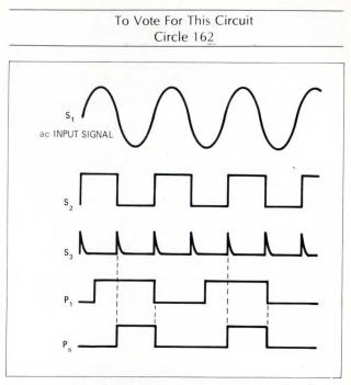
Fig. 2 – **Input signals** ( $S_1$ ) generate zero crossing pulses ( $S_2$ ). Normal enable gate pulses ( $P_1$ ) are then withheld from integrator until zero crossing occurs ( $S_2$ ), at which time the zero-crossing gate ( $P_e$ ) enables the integrator tank circuit.
