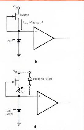
Fig. 2-Reference sources with greatest stability use a constant current source to minimize changes due to  $\Delta V_{IN}$ .
