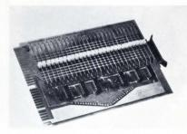
**CONTROL MODULES** 906003 and 906004 make it possible to program additional telephone numbers in any of several combinations. They can be programmed to dial any telephone number up to 14 digits. Models are reprogrammable by means of an unusual slide-bar arrangement. Prices vary from \$60 to \$75 per module, depending on quantity and model desired. G-V Controls Div. of Sola Basic Industries, 101 Okner Parkway, Livingston, NJ 07039.
