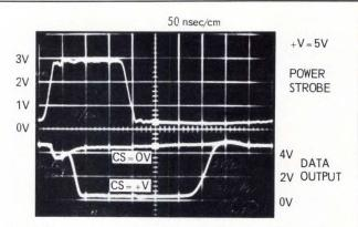
Fig. 5 – **Data output** is HIGH, as shown, when the chip-select line is in the OFF state. However, the voltage decay time of  $V_{cc}$  decreases the recovery time of the data output upon the enabling of the select line.
