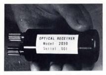
**OPTICAL RECEIVER,** Model 2030, is intended for wide-band communication links and instrumentation systems. It is an all-solid-state unit with a silicon PIN diode as the light-detector element and a 70 MHz band transimpedance amplifier as the gain stage. Spectral response range is 0.4 to 1.1  $\mu$ m. Prices are from \$72 (1-9) to \$64.50 (10-29), with 2 weeks delivery. Optical Communications Technology, Box 262, Goodyear, AZ 85338. **181**
