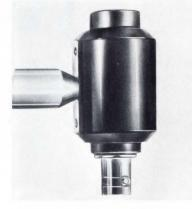
**INFRARED DETECTOR** features response time of <1 nsec. This 10.6 micron detector operates at room temperature and utilizes the photon drag principle. Radiation passing through a doped germanium crystal creates a longitudinal voltage differential which can be monitored by oscilloscope. Oriel Corp. of America, 1 Market St., Stamford, CT 06902. **201**
