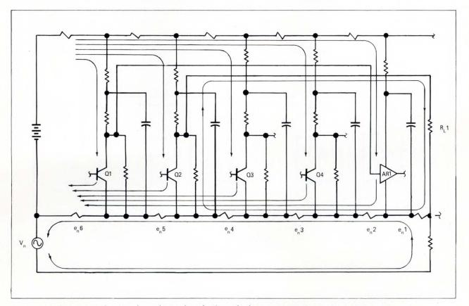
Fig. 1-Typical mass-ground system shows the number of noise paths that can exist. Each stage has both ac and dc paths.
