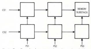
Fig. 6-**Two-dimensional structure** reduces the number of address drivers. Inputs PS1, PS2 and PS3 are separate power strobes and CS1 and CS2 are separate chip selects into the memory array substacks.
