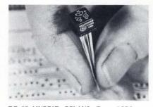
**TO-5<sup>2</sup> HYBRID RELAYS,** Type 3SBS, are available in single- or dual-diode versions. Both versions contain diode chips within the relay enclosure for coil suppression. In addition, the dual version protects against accidental application of reverse polarity. They may be ordered calibrated to either voltage or current standards, and with a choice in headers and coil resistance. General Electric, 777 14th St., N.W. Washington, D C 20005. **184**
