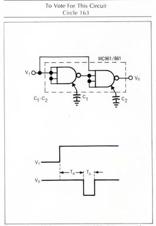
**Monostable multivibrator** uses expandable DTL gates with capacitors connected to expander terminals to provide required delay and pulse width. As shown, leading edge of input pulse triggers the circuit to produce delayed output pulse with delay  $T_d$  and width  $T_p$ .
