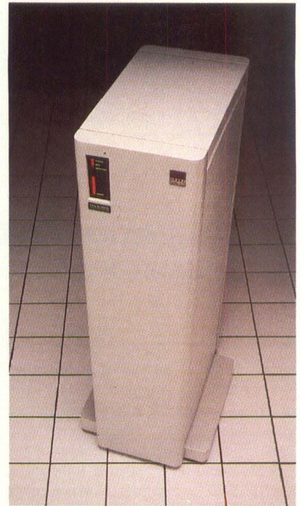
Figure 3: The Mach 1000, a logic simulation accelerator from Silicon Solutions, is built around the CADAT simulation algorithm and includes 10 full custom ICs, a 68010 front-end processor and up to 8 Mbytes of main memory. Special emphasis has been put on developing a compiler that speeds both design flattening and interconnection, and provides incremental compilation.
