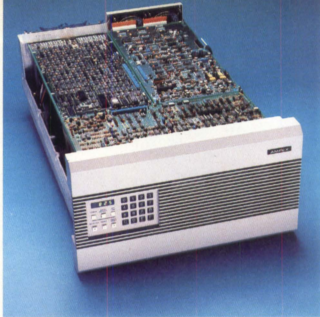
Ampex's 825 14" disk drive uses SMD at 1.859 Mbytes/sec. Models with 330 or 660 Mbytes capacity can be upgraded to 825 Mbytes.
