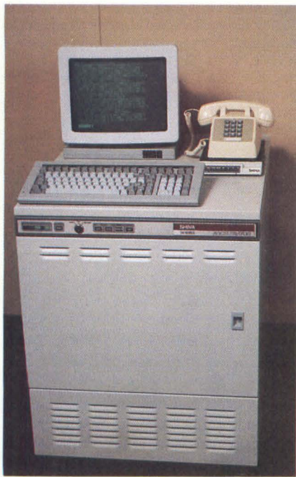
Figure 1: Shiva Multisystems' SX Series SPICE accelerators execute simulations at speeds ranging from 20 to 100 times faster than a VAX 11/780. The machines' performance is a result of PowerSPICE, a relaxation-based SPICE algorithm, and SPICEEngine, a parallel processing number crunching computer. To the circuit designer, the PowerSPICE interface appears identical to traditional SPICE programs.
