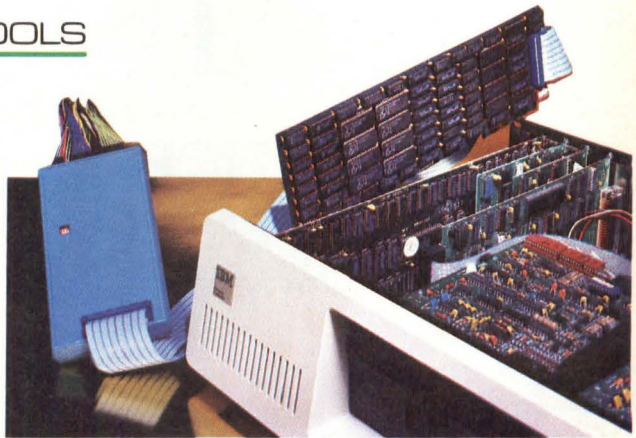
Figure 1: The PCI-4304 logic analyzer from Burr-Brown provides 32 input channels via a plug-in board, 3-foot ribbon cable and instrument pod that extends from the computer to the digital system under test.
