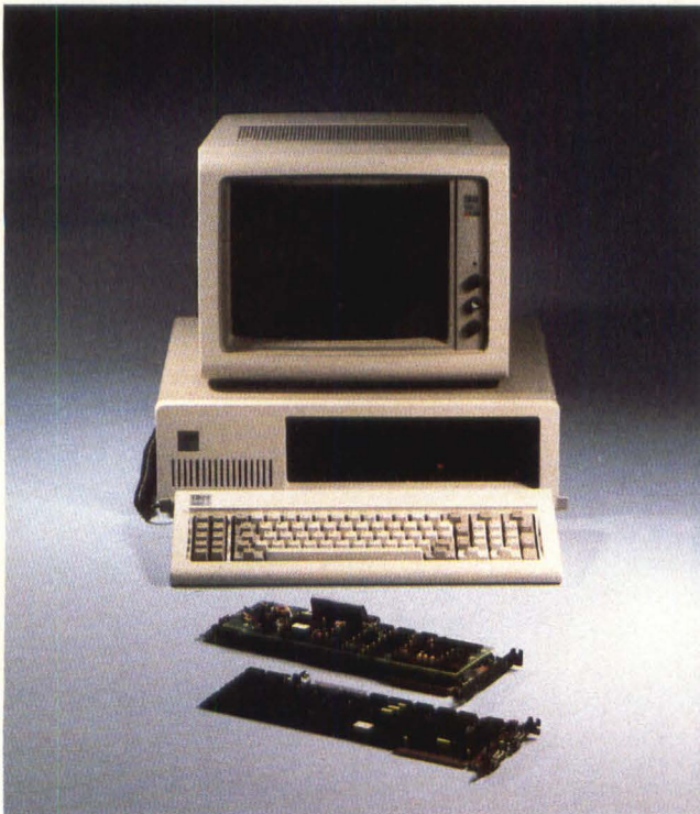
Figure 3: The GraphOver two-board set for the IBM PC from New Media Graphics allows 640 \times 400 graphics to be combined on a video background.
