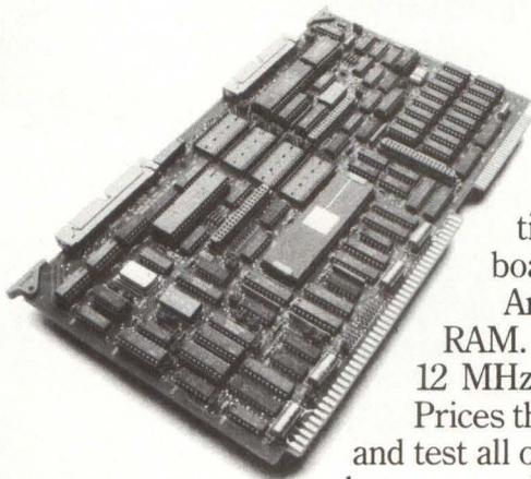
Total Multibus/IEEE 796 compatibility. 10 MHz operation with no wait states. 128K of dual-ported RAM. Two multi-protocol serial I/O ports. Two iSBX Multimodule connectors. One 16-bit triple counter/timer. And one 24-bit parallel port. All on our M68K10 board for \$895 in quantity 100.
