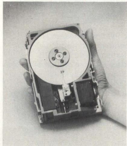
The Model TM362 3 1/2" Winchester disk drive employs a unique closed-loop positioning system and plated media to
