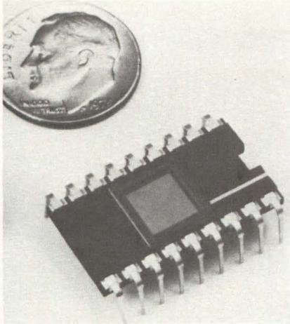
Intended for producing standard interlaced 525-line video with precision image geometry, the SID504 CCD contains 512 vertical × 403 horizontal pixels (206,336 picture elements). It has a spectral response that includes both visible wavelengths between 400 and 700 nm, and wavelengths extending into the near-infrared spectrum to about 1100 nm. **RCA, Lancaster, PA** **Circle 191**
