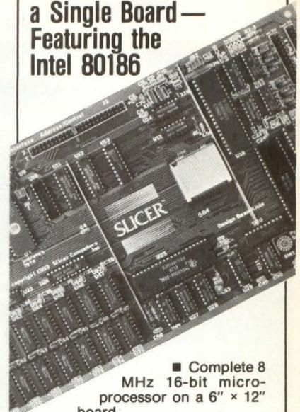
■ Complete 8 MHz 16-bit micro-processor on a 6" x 12" board
