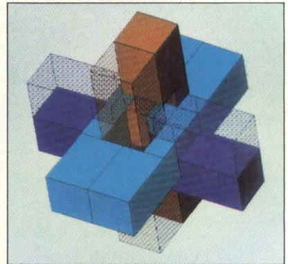
SOLIDVIEW, Lexidata's patented technology for the display of solid models, is available as an option on selected LEX 90 display processors. Its translucent shading pattern allows you to see inside your solid model.
