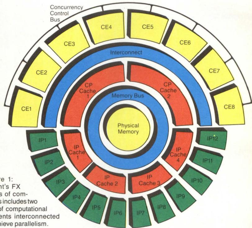
interconnected with each other through a dedicated parallel processing control bus. All of the processors in the complex are applied to the execution of a single program, transparent to the programmer.
