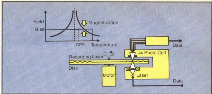
Verbatim uses a thermo-magneto-optical process to store 40 Mbytes on a 3½" disk. A laser temporarily heats a storage film to reduce its coercivity and to permit writing by an external magnetic field. The bits are stored when the film returns to room temperature and its normal high-coercive state. Reading occurs when a beam of polarized laser light shines through the transparent film and a photodetector senses the degree of rotation of the polarized light.
