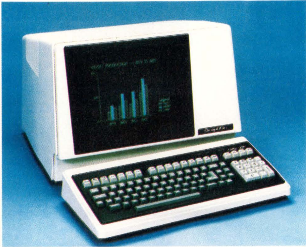
Figure 1: The GraphOn GO-140 integrated alphanumeric/graphics terminal that uses a single-board design.
