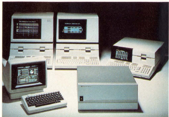
Figure 5: Aydin's AYCAD is a 8086/8087 based generalized CAD workstation initially targeted for VLSI design, but intended to provide users with a low cost entry system for workstation applications.
