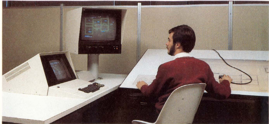
Figure 5: Aydin's AYCAD is a 8086/8087 based generalized CAD workstation initially targeted for VLSI design, but intended to provide users with a low cost entry system for workstation applications.
