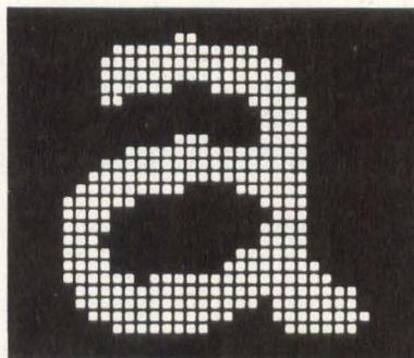
**Fig 1** The OCR changes alphanumeric into a pattern of dots, and sends them to the video buffer, which circumscribes a rectangular box around each element.
