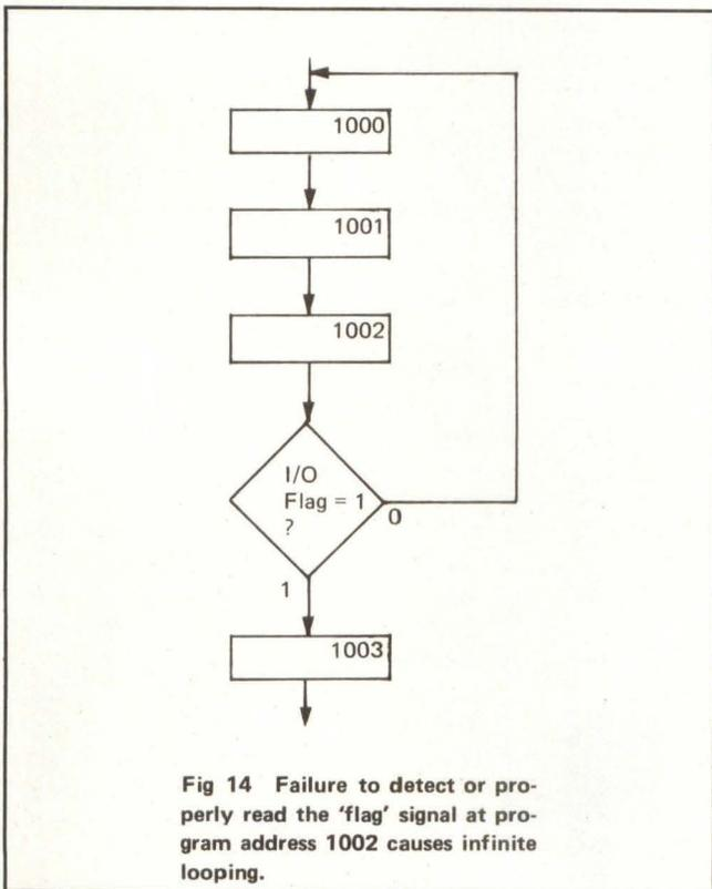
**Fig 14** Failure to detect or properly read the 'flag' signal at program address 1002 causes infinite looping.
