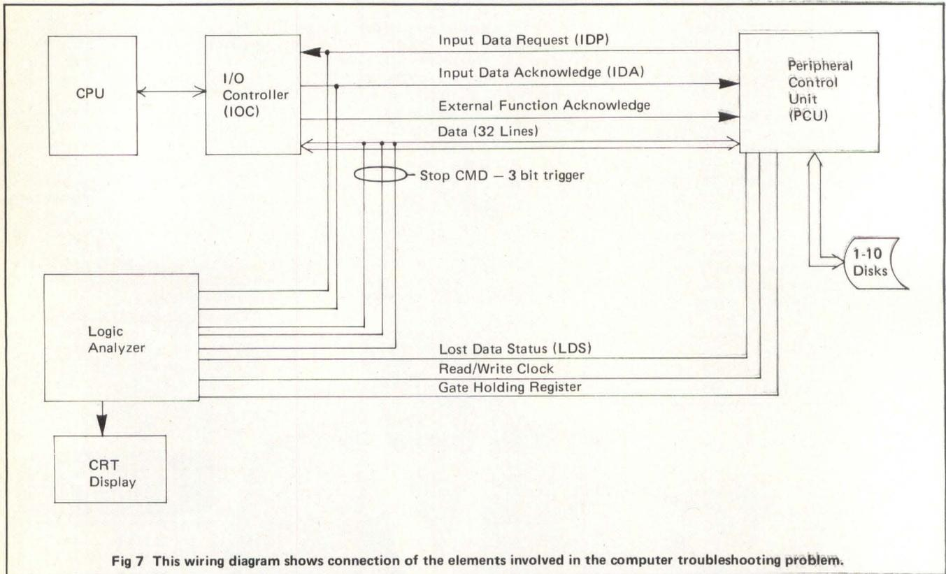
Fig 7 This wiring diagram shows connection of the elements involved in the computer troubleshooting problem.
