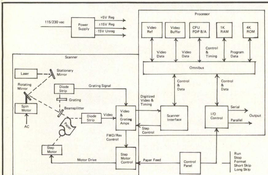
**Fig 2** The block diagram above illustrates the operation of the OCR. The step motor moves the paper in 0.004" increments; after the laser scanner detects characters, it sends the digitized picture elements to the PDP-8/A's video buffer. There, the characters are boxed and identified, or accepted as a best guess.
