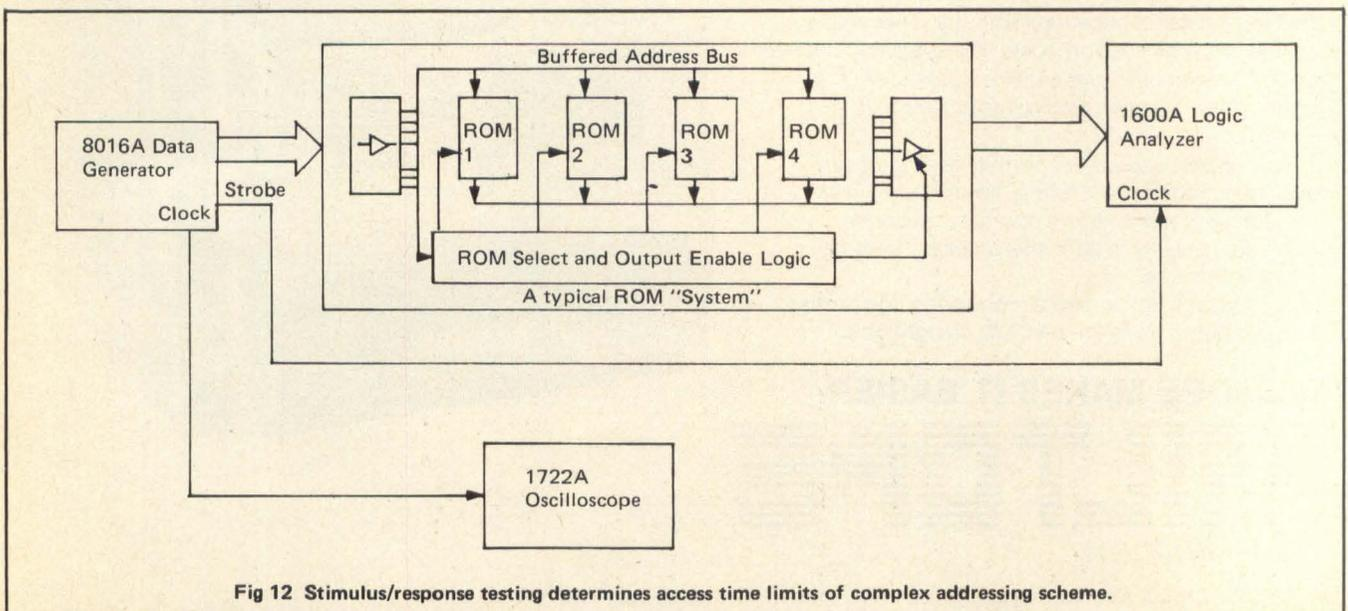
Fig 12 Stimulus/response testing determines access time limits of complex addressing scheme.
