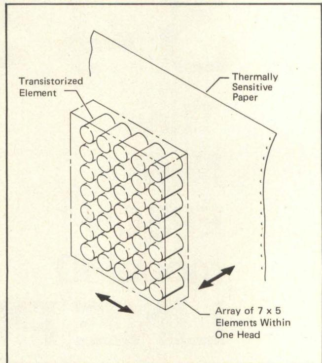
Fig 10 A single thermal matrix head moves across the paper and stops momentarily at each character position. The matrix head elements are transistors that when switched on produce heat. The hot spots force a heat sensitive dye in the paper to change color and create a series of dots.
