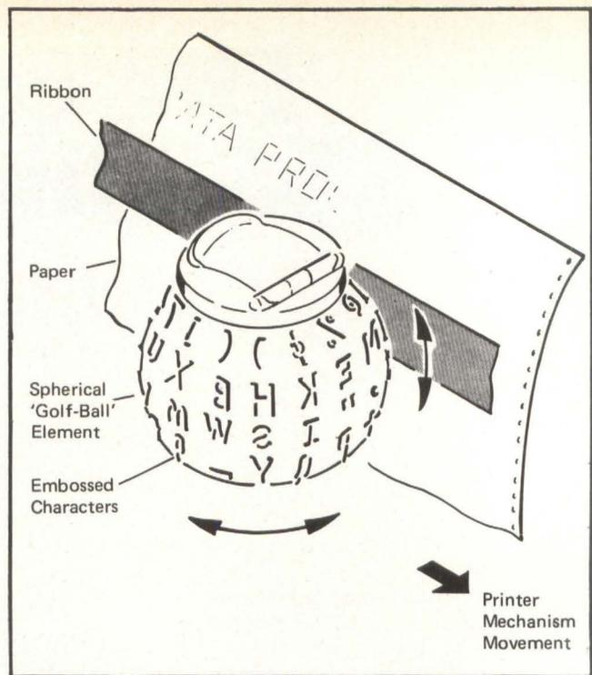
**Fig 3** Golf ball printing mechanism performs its printing functions much as the cylinder mechanism, except that the sphere itself strikes the paper without the aid of a hammer.
