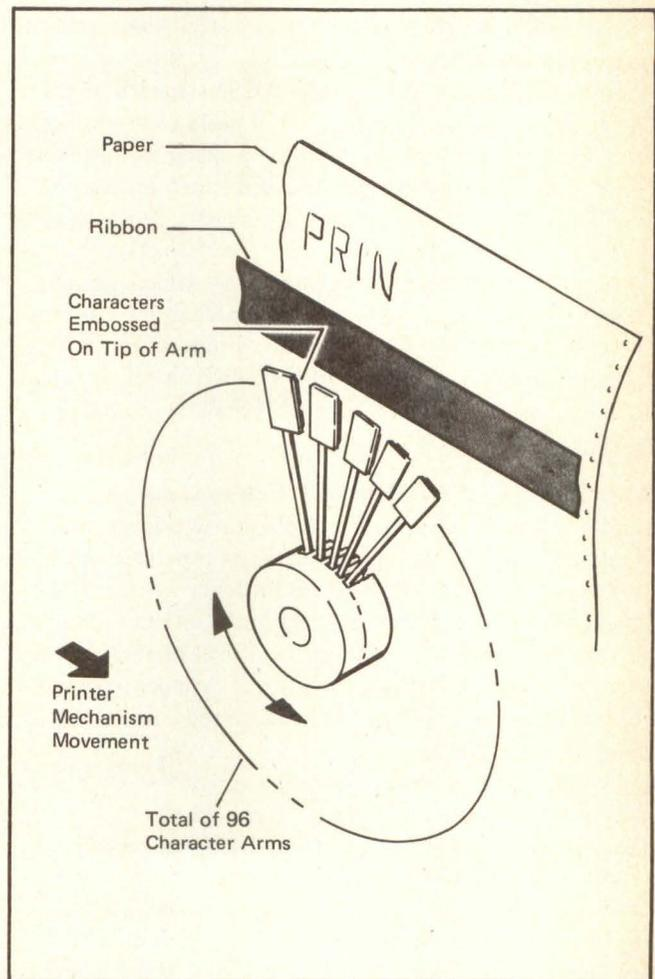
**Fig 4** Daisy wheel printing element consists of a series of "petals" with a single character at each tip. After the wheel moves into position along the paper and rotates to locate the appropriate character, a hammer strikes the petal tip. A variant (not shown), the cup wheel, is shaped like a tulip. It operates on the same principle, but rotates about a vertical rather than horizontal axis.
