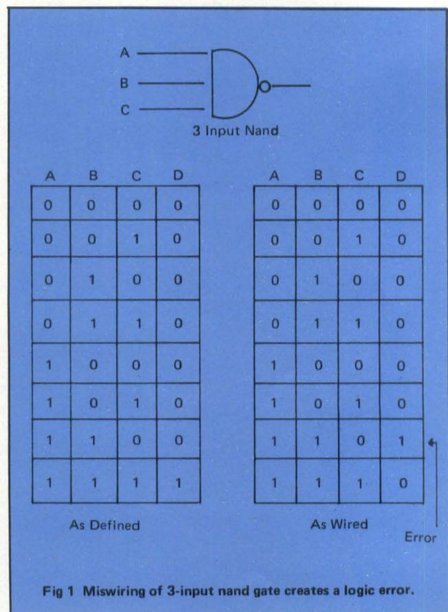
Fig 1 Miswiring of 3-input nand gate creates a logic error.
