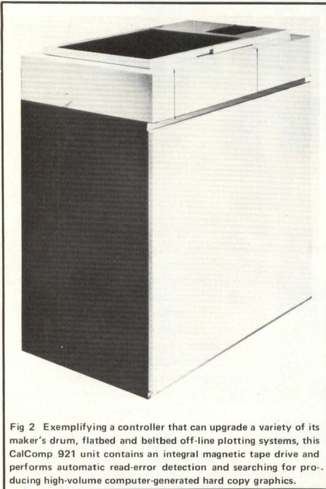
**Fig 2** Exemplifying a controller that can upgrade a variety of its maker's drum, flatbed and beltbed off-line plotting systems, this CalComp 921 unit contains an integral magnetic tape drive and performs automatic read-error detection and searching for producing high-volume computer-generated hard copy graphics.
