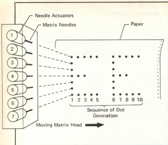
**Fig 8** Serial matrix printers employ a single head that moves across the page. Electromagnetically driven pins in the head form the characters from dot patterns. Each scan of the print head across the page produces one line of print. The number of pins varies, but 7 is most common.
