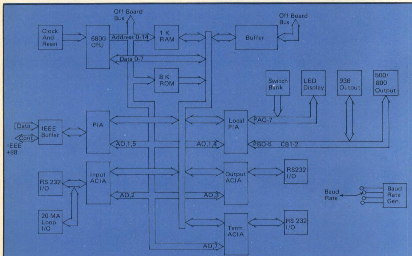
**Fig 1** Simplified block diagram of CalComp Model 906 on-line controller indicates how it can provide significant flexibility for plotters. Off-board buses permit memory expansion, additional I/O circuitry, or greater microprocessing power. The bank of switches provides the operator with a means of setting parameters that define plotter type, information about I/O message headings, parity or other checking code, and a powerful self-analysis and checking capability.
