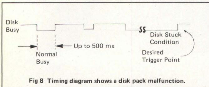
Fig 8 Timing diagram shows a disk pack malfunction.
