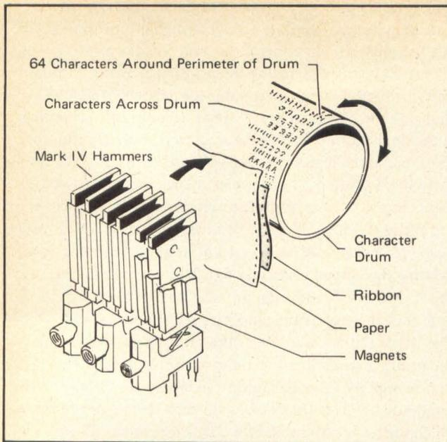
Fig 5 Embossed with a complete character set for each column to be printed, the drum rotates at constant speed. A hammer for each column fires at the precise time to catch the appropriate character beneath it when it strikes.
