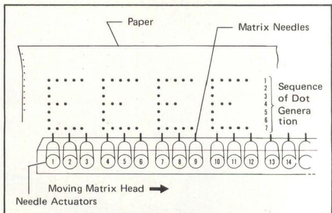
**Fig 9** Matrix comb printers contain several single-element heads housing pins driven by electromagnets. The comb moves back and forth. Each oscillating motion produces a portion of every character in every column. The number of movements required to produce a complete line depends upon character vertical resolution.
