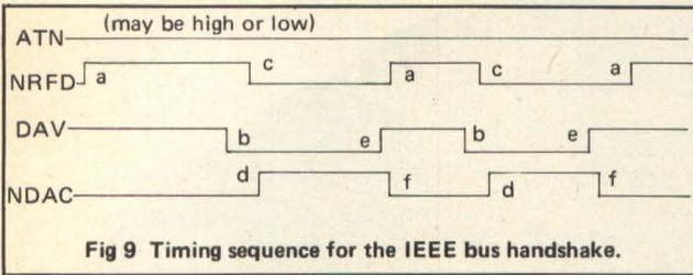
Fig 9 Timing sequence for the IEEE bus handshake.
