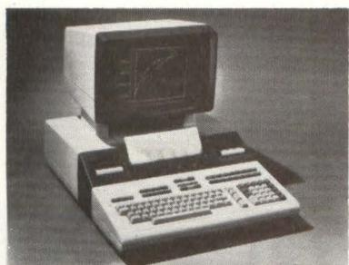
**Fig 1** The Hewlett-Packard System 45 has the most powerful central processor and the largest mass memory ever offered in a desktop computer and incorporates a 12" CRT display, enhanced Basic, applications software and an optional graphics package with high-speed hard-copy printing.
