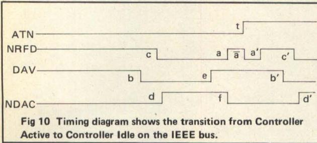
Fig 10 Timing diagram shows the transition from Controller Active to Controller Idle on the IEEE bus.
