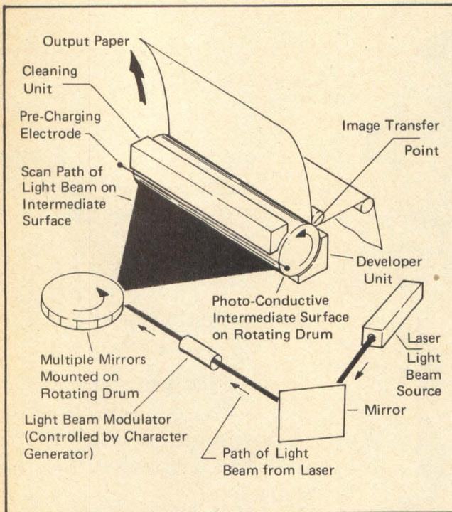
Fig 13 Indirect electrostatic (laser) printers need no special paper. A modulated laser light beam, aimed at an intermediate surface (drum), forms dot matrix characters photoelectrically. The drum is then toned with ink powder and transfers the ink to the paper. Heat fuses the ink to the paper.
