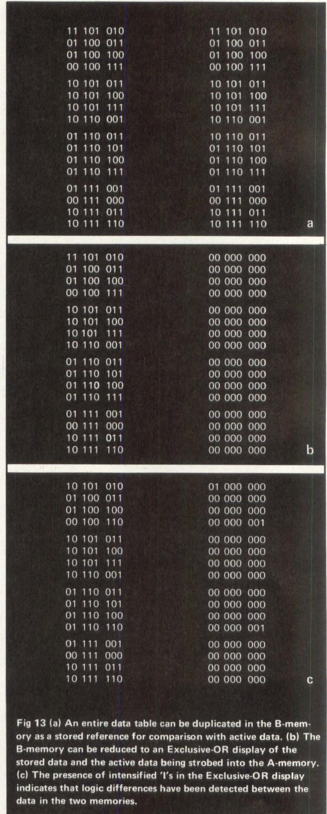
Fig 13 (a) An entire data table can be duplicated in the B-memory as a stored reference for comparison with active data. (b) The B-memory can be reduced to an Exclusive-OR display of the stored data and the active data being strobed into the A-memory. (c) The presence of intensified '1's in the Exclusive-OR display indicates that logic differences have been detected between the data in the two memories.
