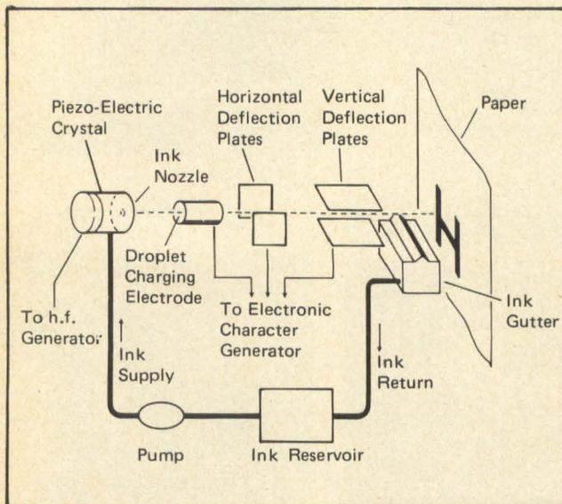
Fig 14 Ink jet printers use a special ink which is charged and directed against plain paper. Electric fields direct the ink against the paper to specific points to form matrix characters. At those points that require no mark, the ink is deflected down into the gutter.
