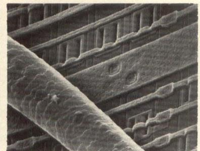
**Fig 3** Using VMOS technology, computer memory transistors are so small that eight of them on an integrated circuit (bottom) will fit in the cross section of a human hair (top).
