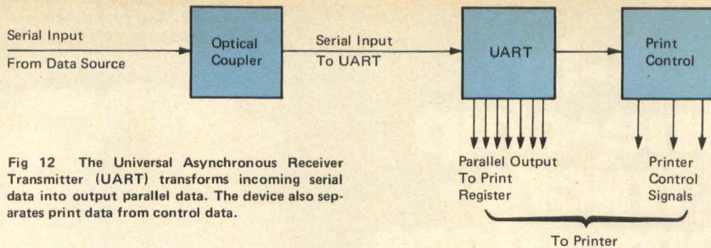
Fig 12 The Universal Asynchronous Receiver Transmitter (UART) transforms incoming serial data into output parallel data. The device also separates print data from control data.
