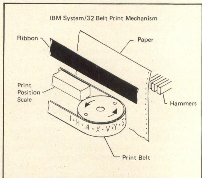
Fig 6 This printing character belt moves at constant speed. Precisely timed hammers make the impressions. The hammer may strike the belt or the paper.
