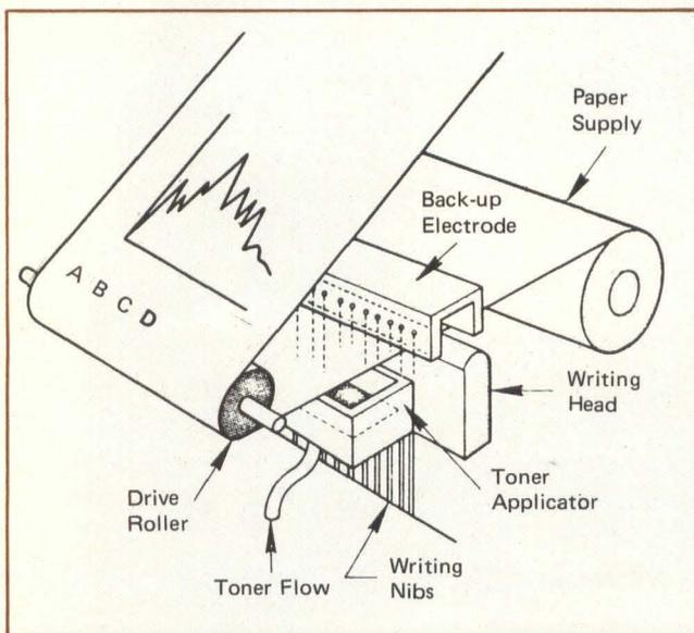
**Fig 11** Direct electrostatic printers use a specially-coated paper passing over an array of styli or nibs. Each stylus is charged to produce the required output. The paper then passes through a toner bath from which the charged areas attract ink particles.
