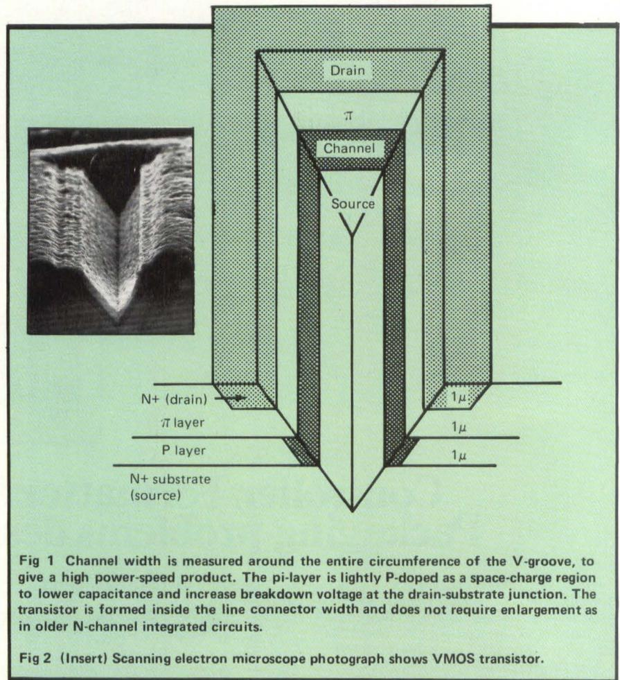
Fig 1 Channel width is measured around the entire circumference of the V-groove, to give a high power-speed product. The pi-layer is lightly P-doped as a space-charge region to lower capacitance and increase breakdown voltage at the drain-substrate junction. The transistor is formed inside the line connector width and does not require enlargement as in older N-channel integrated circuits.
