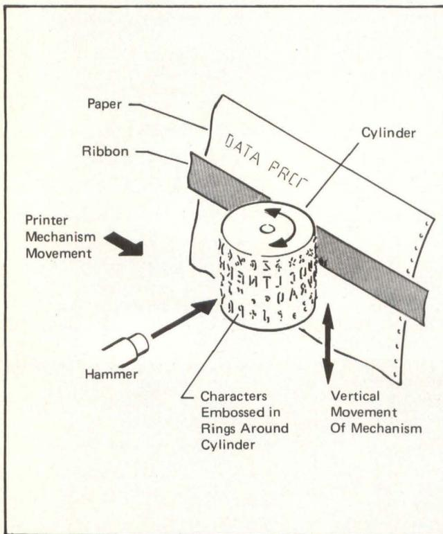
**Fig 2** Part of a cylinder printing mechanism consists of a complete character set embossed in a series of rings around the small cylinder. To print, the mechanism moves the cylinder into position along the paper, rotates it and shifts it vertically, then strikes it with a hammer.
