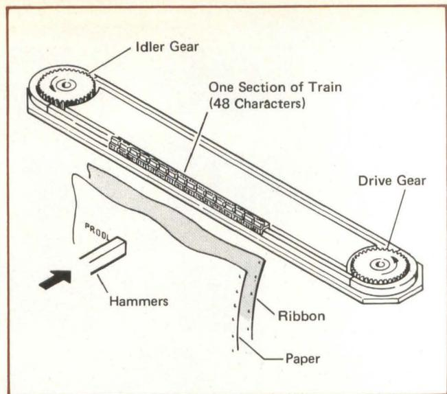
**Fig 7** Similar to a belt machine, the train printer consists of a series of linked character "slugs" moving at constant speed. Precisely timed hammers make the impression striking from behind the paper.
