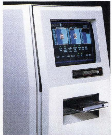
Fault tolerant features are available in several configurations, including automatic bad-sector managements, which is standard with all 1776 subsystems; mirrored disks; redundant subsystem electronics; and redundant computers.
