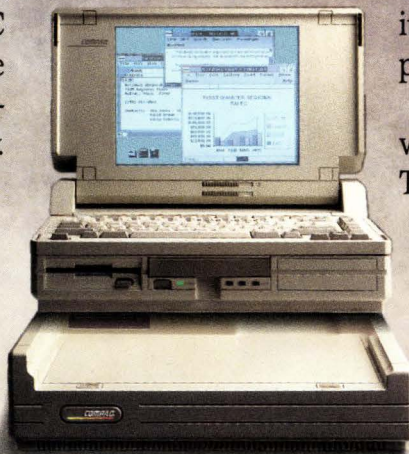
The COMPAQ SLT/286 snaps into an optional Desktop Expansion Base for office use.
