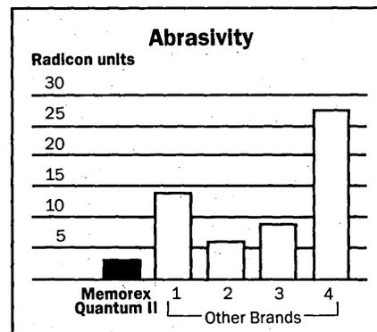
Radicon Test measurements above are obtained by running different computer tapes over an irradiated tape drive head. The higher the count of irradiated particles rubbed onto the tape, the more abrasive the tape.
