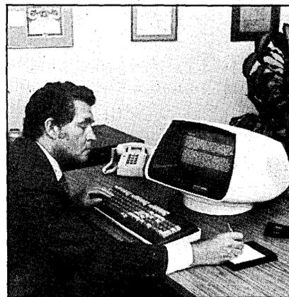
vendor's computers, the terminals display the upper- and lower-case ASCII characters formed in a 7 x 11 dot matrix cell; the display screen has a capacity of 24 lines of 80 characters. Both terminals have typewriter-style keyboards and 14-key numeric clusters; additionally, the D200 has a 12-key screen management keypad, and a 15-key function keypad. A subset of D200 func-
