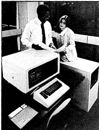
A typical 5280 configuration, consisting of a 64KB programmable display station, two diskette drives (1.2MB each), a 120cps 5256 serial printer, and a communications adaptor, leases for \$517 a month over two years; this configuration sells for \$16,660. Depending on configuration and quantity, 5280 pricing begins at \$166 a month (for two-year leases) and \$5,630 for purchase. Shipments are scheduled to begin in June. INTERNATIONAL BUSINESS MACHINES CORP., General Systems Div., Atlanta, Ga.
