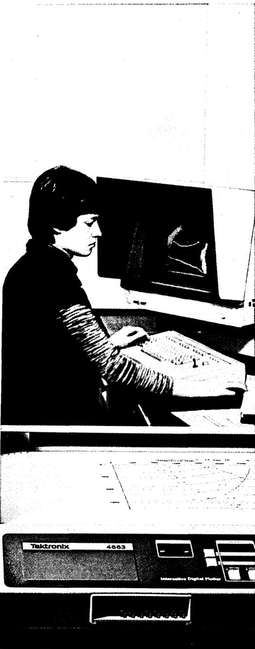
graphics equipment lets us digitize each rock layer configuration in seconds so we can quickly test concepts of what's going on in the earth."
