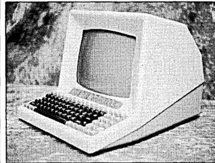
dard. The minimAS communicates via an RS232 interface at speeds of up to 19.2Kbps; a 20mA current loop interface is optional. An auxilliary printer port is standard equipment. In lots of 100, the minimAS sells for \$499. MICRO APPLICATIONS SYSTEMS, INC., Minneapolis, Minn.
