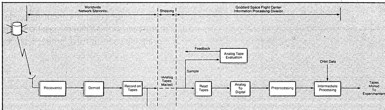
Fig. 1. Previous system for collecting and processing satellite data.
