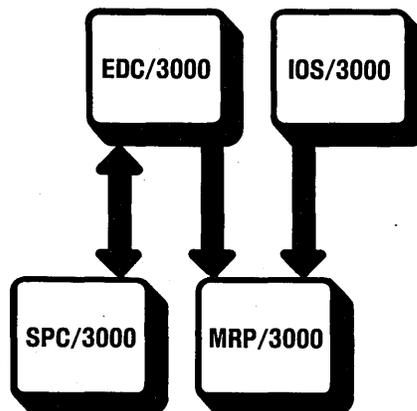
**MRP/3000**, Material Requirements Planning, simulates the complex flow of material necessary to meet a production schedule.
