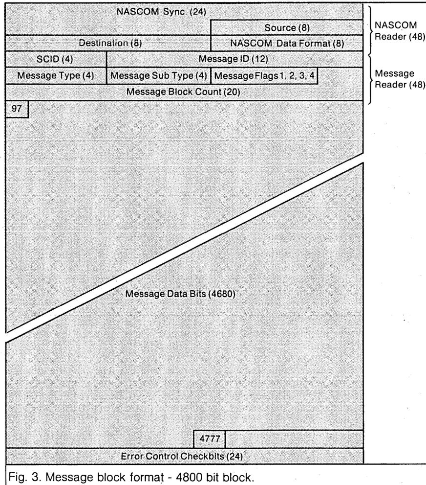
Fig. 3. Message block format - 4800 bit block.
