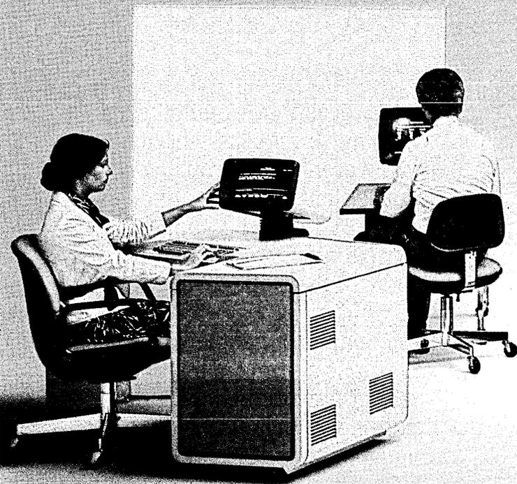
**HP 250** The HP 250 is a powerful small business computer that has a typewriter-like keyboard and an adjustable video screen with eight programmable "soft keys" to make the user feel right at home. Priced from \$23,500, the HP 250 can support five local terminals and even act as a terminal for the HP 3000.
