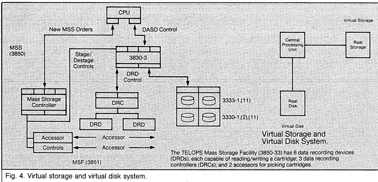
Fig. 4. Virtual storage and virtual disk system.
