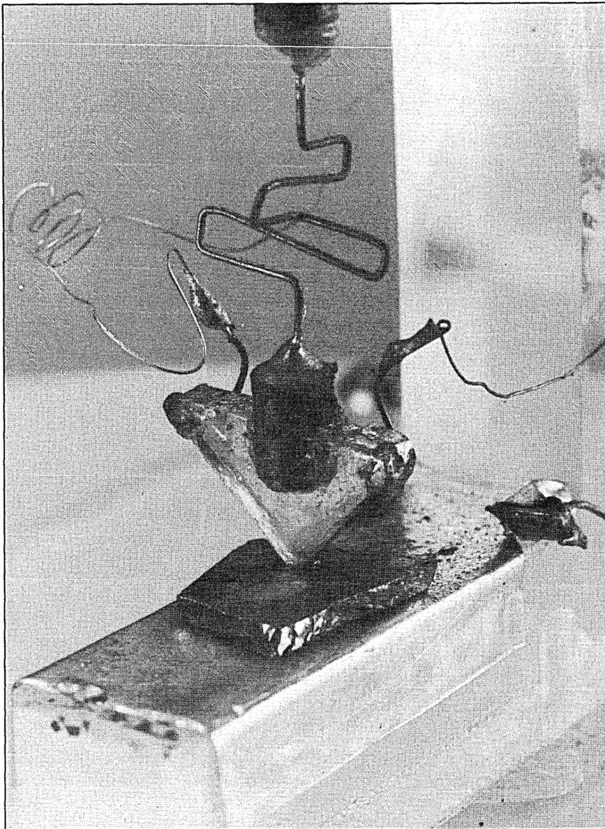
This first transistor, a "point-contact" device, amplified electrical signals by passing them through a tiny bit of germanium, basically the same operation performed by today's silicon junction transistors. (Photo courtesy of Bell Labs.)
